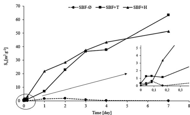
Fig. 2 Specific surface area  $S_a$  [m<sup>2</sup> g<sup>-1</sup>] of the glass materials during exposure to SBF-Ø, SBF+T and SBF+H solutions (with detail).
