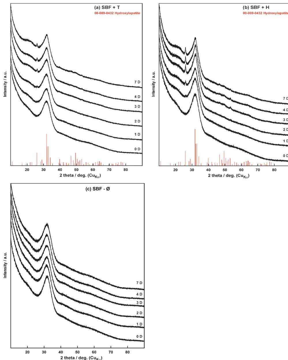
Fig. 8 Diffractograms of glass materials before (0D) and during interaction (1–7D) in the solutions: (a) SBF+T, (b) SBF+H, (c) SBF-Ø.
