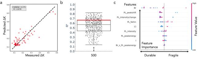
Fig. 3 (a) Parity plot of an RFR model yielding a modal  $R^2$  goodness-of-fit metric. (b) Box plot of the 500 iterations of the 5-fold cross-validated model. Mode shaded in red. (c) SHAP table for the mode  $R^2$  model produced in this study.
