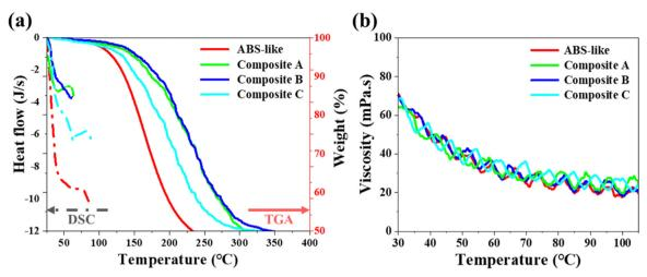
Fig. 4 (a) Thermal analysis of ABS-like resin and composites A, B and C with TGA (solid line) and DSC (dashed line). (b) Rheology test on ABS-like and composites A, B and C.
