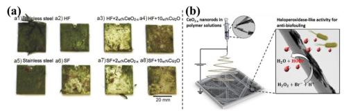
Fig. 3 (a) Selected samples after seven and half weeks of the static field immersion.<sup>14</sup> Reproduced from ref. 14 with permission from Wiley, copyright 2017. (b) Fabrication of CeO<sub>2-x</sub> nanofibrous mats by electrospinning. 43 Reproduced from ref. 43 with permission from ACS, copyright 2018.
