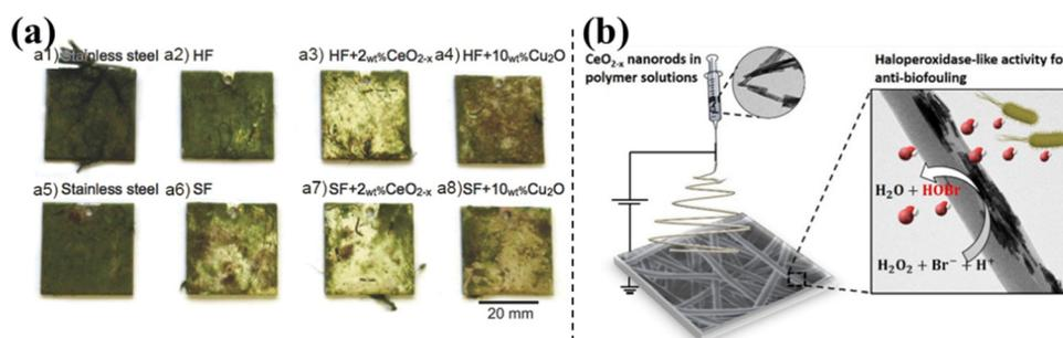
Fig. 3 (a) Selected samples after seven and half weeks of the static field immersion.<sup>14</sup> Reproduced from ref. 14 with permission from Wiley, copyright 2017. (b) Fabrication of  $CeO_{2-x}$  nanofibrous mats by electrospinning.<sup>43</sup> Reproduced from ref. 43 with permission from ACS, copyright 2018.
