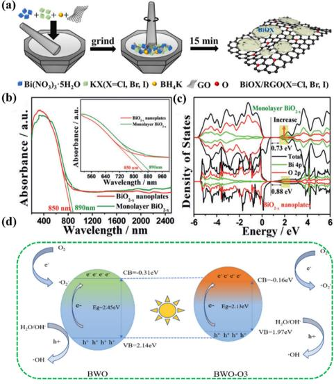
Fig. 3 (a) Synthesis of the BiOX/RGO (X = Cl, Br and I) composite. 6 Copyright 2021, Elsevier. (b) UV/vis-NIR DRS of BiO $_{2-x}$ . (c) Total density of states (TDOS) of BiO<sub>2-x</sub>. <sup>68</sup> Copyright 2017, Wiley. (d) Schematic of Bi<sub>2</sub>WO<sub>6</sub> with/without oxygen vacancies. <sup>69</sup> Copyright 2023, Elsevier.
