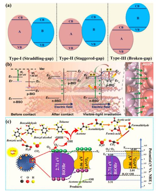
Fig. 4 (a) Schematic of three types of heterojunctions. Ropyright 2021, Elsevier. (b) Schematic of the BiOI/Bi<sub>2</sub>O<sub>2</sub>SO<sub>4</sub> heterojunction. Popyright 2021, Elsevier. (c) Schematic of the BiOI/Bi<sub>2</sub>O<sub>2</sub>SO<sub>4</sub> heterojunction. Elsevier. (c) Schematic of the bandgap match of 3% LaVO<sub>4</sub>/BiOBr and the degradation pathway of gaseous acetone or toluene. 80 Copyright 2020, Elsevier.
