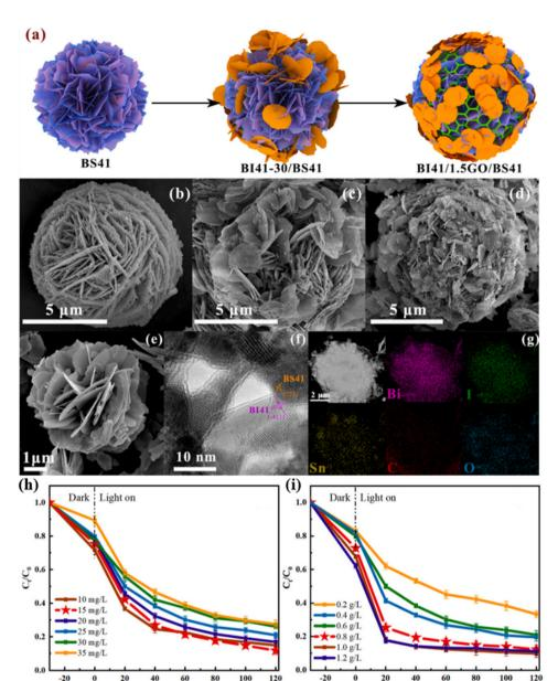
Fig. 5 (a) Schematic of the synthesis process of the BI41/1.5GO/BS41 ternary composite photocatalyst; SEM images of (b) BS41, (c) BI41–30/BS41, and (d) BI41/1.5GO/BS41, and (e) BI41. (f) HRTEM images and (q) element mapping distribution of BI41/1.5GO/BS41. (h) and (i) Degradation curve of TC with different concentrations of BI41/1.5GO/BS41 under illumination. <sup>128</sup> Copyright 2023, Elsevier.
