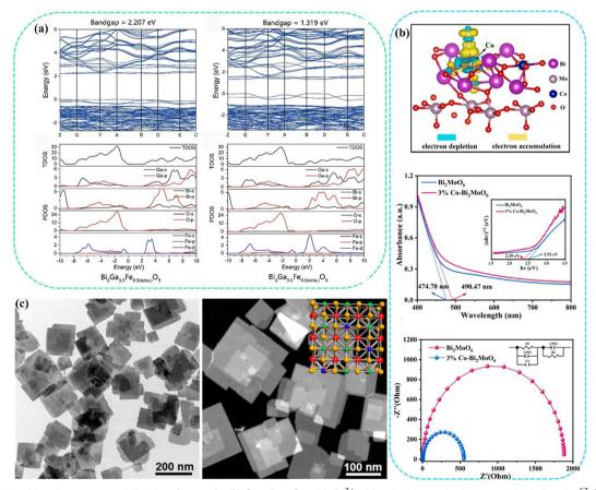
Fig. 2 (a) Calculated band structure and density of states for  $Bi_2Ga_{3.5}Fe_{0.5}O_9$  with  $Fe^{3+}$ , either in the tetrahedral or octahedral cavity. <sup>53</sup> Copyright 2017, Elsevier. (b) Differential charge densities of Co-Bi<sub>2</sub>MoO<sub>6</sub>, UV-vis DRS spectra and ElS of Bi<sub>2</sub>MoO<sub>6</sub> and 3% Co-Bi<sub>2</sub>MoO<sub>6</sub>.  $^{55}$  Copyright 2023, Elsevier. (c) TEM images of BiOCl and BiOCl NSs-Fe-5%. 56 Copyright 2019, American Chemical Society.
