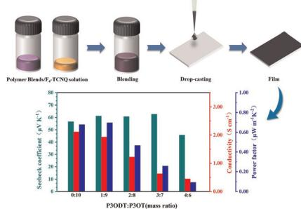
**Electrical and thermoelectric properties of a poly(3-(2-octyldodecyl)thiophene)/poly(3-octylthiophene)/2,3,5,6-tetrafluoro-7,7',8,8'-tetracyanoquinodimethane viscoelastic polymer blend doping system**
