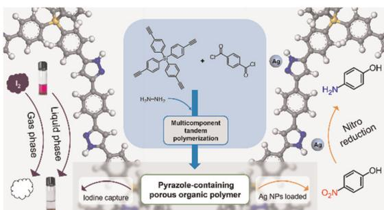
**Multicomponent tandem polymerization for the preparation of a pyrazole-containing porous organic polymer for iodine capture and the nitro reduction reaction**
