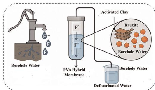
**Defluorination of borehole water using activated clay and bauxite-laden polyvinyl alcohol hybrid membranes**
