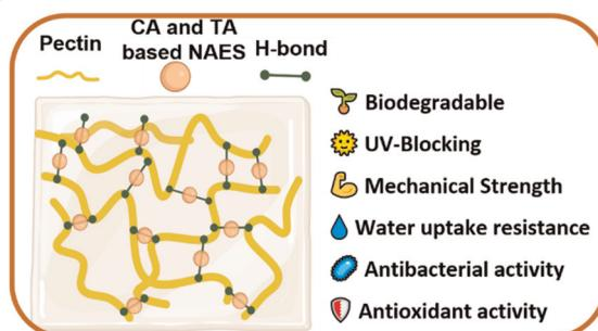
**Fabrication of biodegradable and active pectin-based films with enhanced properties by the incorporation of natural eutectic solvents**
