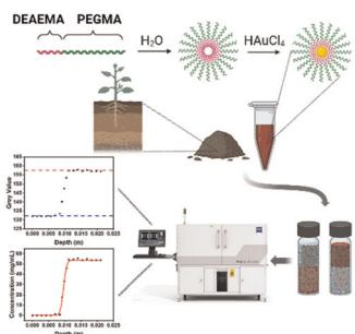
**A micelle-templated nanoparticle contrast agent enables dynamic microscale X-ray computed tomography imaging of the soil aqueous phase**
