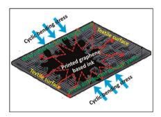
Interfacial stress transfer in graphene-based polymeric inks on a textile surface for long term cycling stability
