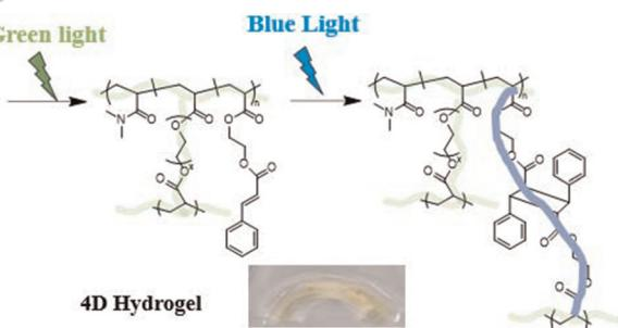
**Preparation of 4D hydrogels with PET-RAFT and orthogonal photo-reactions**
