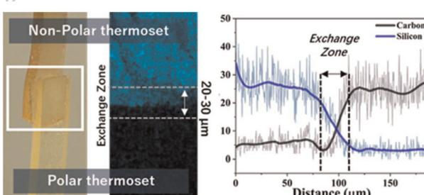
**Adhesive-less bonding of incompatible thermosetting materials**
