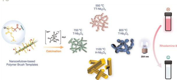
**Nanostructuring niobium oxides using polymer-grafted cellulose nanocrystals and nanofibers as sacrificial scaffolds**
