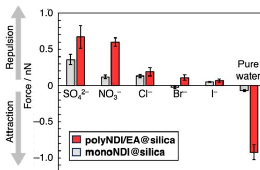
**Fig. 4** Force detected on **polyNDI/EA@silica** and **monoNDI@silica** using force curve measurements in pure water or aqueous solutions of TBA<sub>2</sub>SO<sub>4</sub>, TBANO<sub>3</sub>, TBACl, TBABr, or TBAI.
