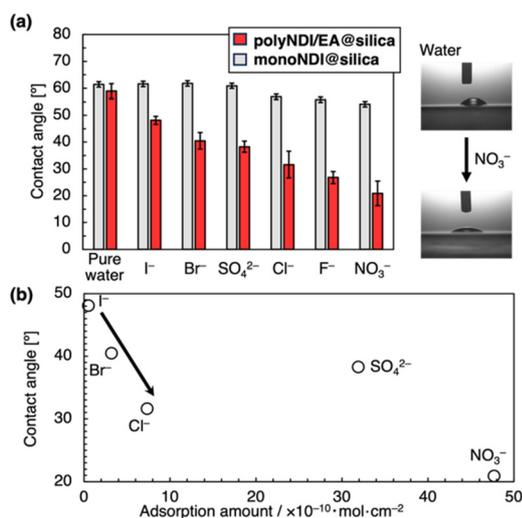
**Fig. 5** (a) Contact angles of **polyNDI/EA@silica** and **monoNDI@silica** for pure water and aqueous solutions of  $\text{Na}_2\text{SO}_4$ ,  $\text{NaNO}_3$ ,  $\text{NaF}$ ,  $\text{NaCl}$ ,  $\text{NaBr}$ , and  $\text{NaI}$ , and photographs of pure water and aqueous solution of  $\text{NaNO}_3$ . The concentration of the sodium salts was fixed at 10 mM. (b) Contact angle vs. adsorption amount of anions.
