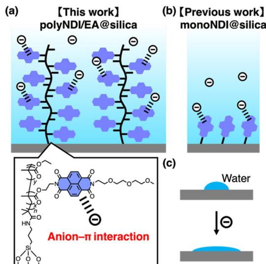
**Fig. 1** Anion- $\pi$  interaction at water/solid interfaces using NDI-modified polymer brush (**polyNDI/EA@silica**) and monolayer (**monoNDI@silica**) (a and b). Enhancement of water wettability of the solid surface with anions in aqueous solutions (c).
