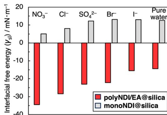
**Fig. 6** Interfacial free energies of **polyNDI/EA@silica** and **monoNDI@silica** for pure water and aqueous solutions of  $\text{Na}_2\text{SO}_4$ ,  $\text{NaNO}_3$ ,  $\text{NaCl}$ ,  $\text{NaBr}$ , and  $\text{NaI}$  according to contact angle measurements.
