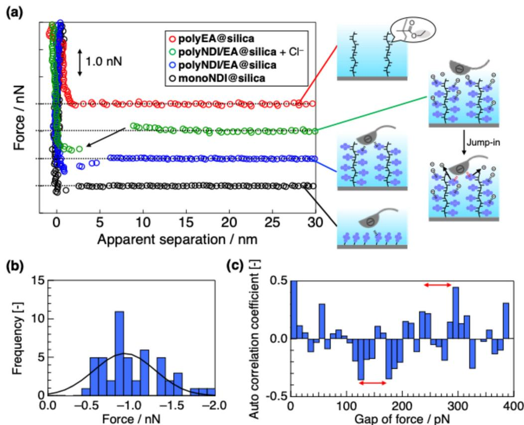
**Fig. 3** (a) Approaching force curves of **polyEA@silica** in pure water, **polyNDI/EA@silica** in pure water or aqueous 10 mM TBACl solution, and **monoNDI@silica** in pure water (from top to bottom). The Z-scale interval was 1.0 nN. (b) Histogram of the observed attractive force on the NDI-modified polymer brush in pure water in pure water ( $n = 100$ ) and (c) its autocorrelation coefficient.
