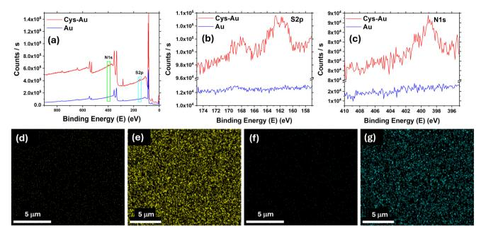
Fig. 2 (a-c) XPS (a) survey spectra, (b) S 2p and (c) N 1s spectra of bare Au (blue) and Cys on Au (Cys-Au, red) substrates. (d-q) SEM-EDX images showing the elemental mapping of sulfur: on Au (d) and Cys-Au (e); nitrogen: on Au (f) and (g) Cys-Au.
