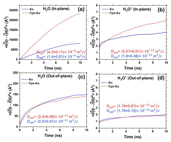
Fig. 7 Mean square displacement of water and hydronium (H<sub>3</sub>O<sup>+</sup>) ions in Nafion films on Au and Cys-Au: (a) water, in-plane; (b) H<sub>3</sub>O<sup>+</sup> ions, inplane; (c) water, out-of-plane; (d) H<sub>3</sub>O<sup>+</sup> ions, out-of-plane. Corresponding self-diffusion coefficients (D<sub>self</sub>) of species in a certain direction are shown in insets.
