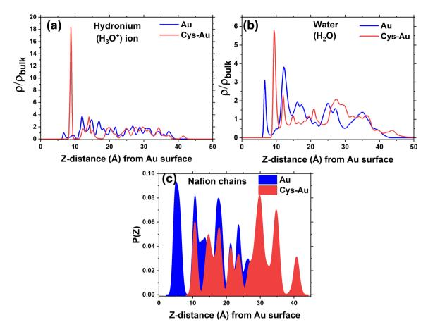
Fig. 6 Normalized density distribution of (a) hydronium (H<sub>3</sub>O<sup>+</sup>) ion and (b) water (H<sub>2</sub>O) for Nafion on Au and Cys-Au. (c) Probability distribution of Nafion chains with the z-distance from the substrate.
