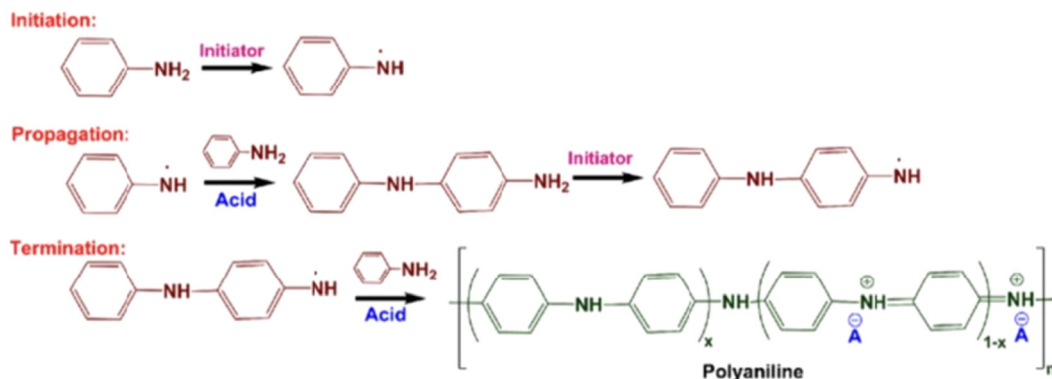
Fig. 4 Chemical polymerization mechanisms of polyaniline. Chemical polymerization of polyaniline is carried out in acidic medium by using a common initiator such as ammonium persulfate and potassium persulfate. 99 Reproduced with permission from ACS.
