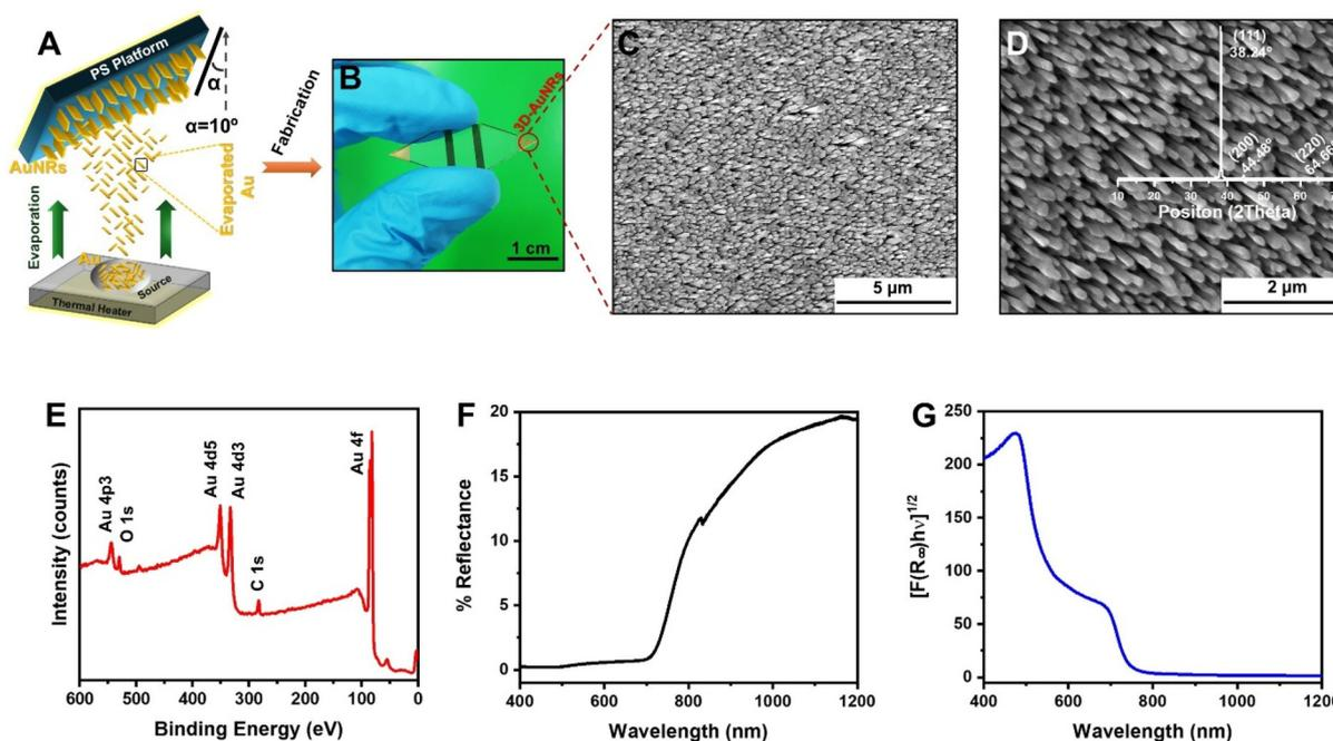
**Fig. 5** Schematic illustration of the fabrication process of 3D-AuNR assemblies on a PS platform (A). Optical image of a fabricated PS platform with 3D-AuNR assemblies (B). SEM images of 3D-AuNR assemblies on a PS platform (C and D) (inset shows the XRD pattern of AuNR assemblies deposited on the PS platform). XPS spectrum of 3D-AuNR assemblies deposited PS platform (E). UV-Vis reflectance spectrum (F) and Kubelka–Munk function (G) of 3D-AuNR assemblies deposited PS platform.
