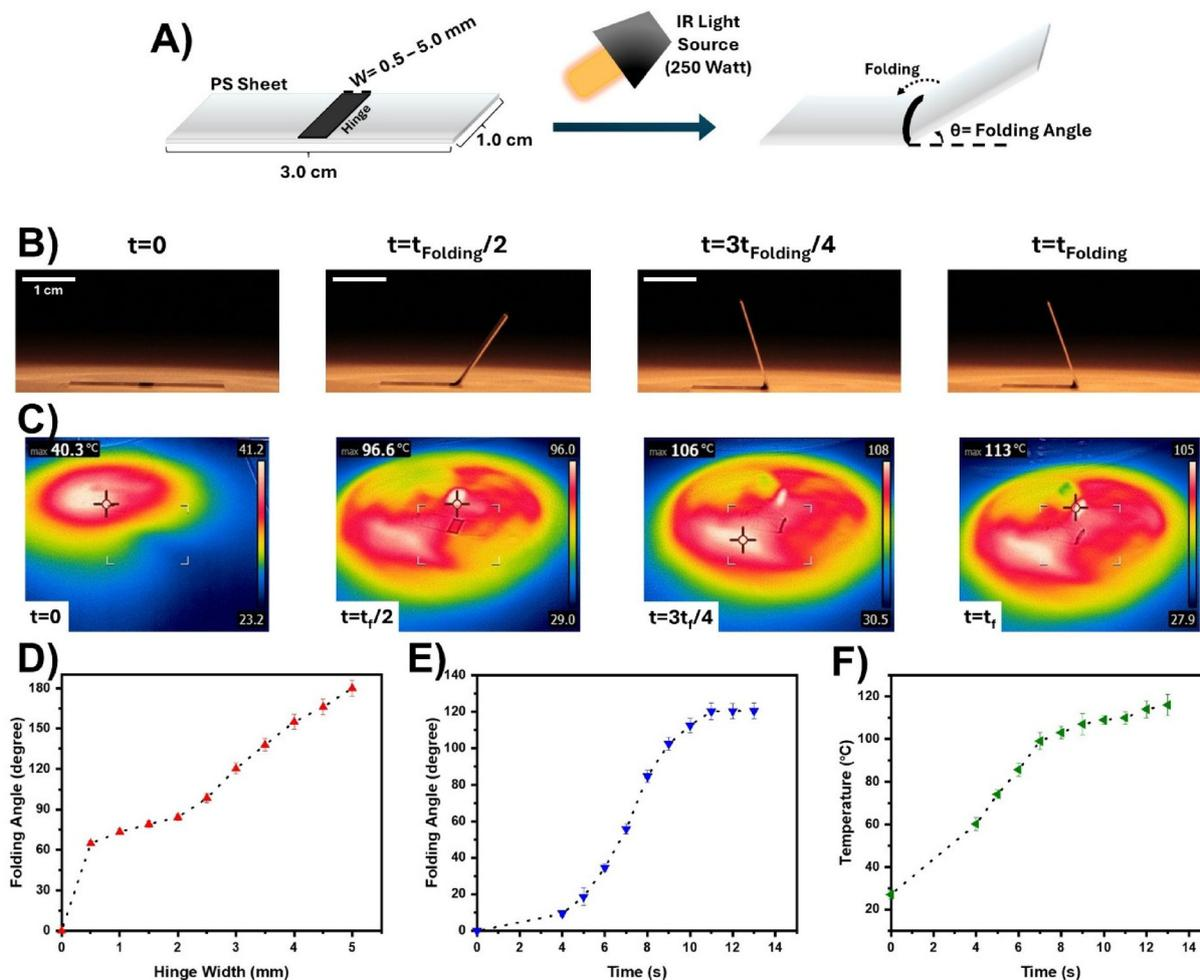
**Fig. 1** Schematic illustration of the fabrication and folding process of a PS platform (A). Optical (B) and thermal camera (C) images of a 2D PS platform with a black colored hinge (3.0 mm width) under IR light illumination (250 W). Folding angles of 2D PS platforms as a function of hinge width (D). Folding angles of 2D PS platforms with a 3.0 mm hinge width as a function of time (E), and temperature changes on a PS platform under IR light illumination as a function of time (F).
