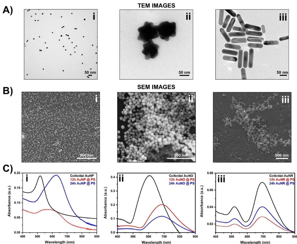
**Fig. 3** TEM images of synthesized colloidal AuNPs (i), AuNOs (ii), and AuNRs (iii) (A). SEM images of the AuNP- (i), AuNO- (ii), and AuNR- (iii) decorated PS platforms for 24 h retention time periods (B). UV-vis spectra of AuNP- (i), AuNO- (ii), and AuNR- (iii) decorated PS platforms with different retention time periods (C).
