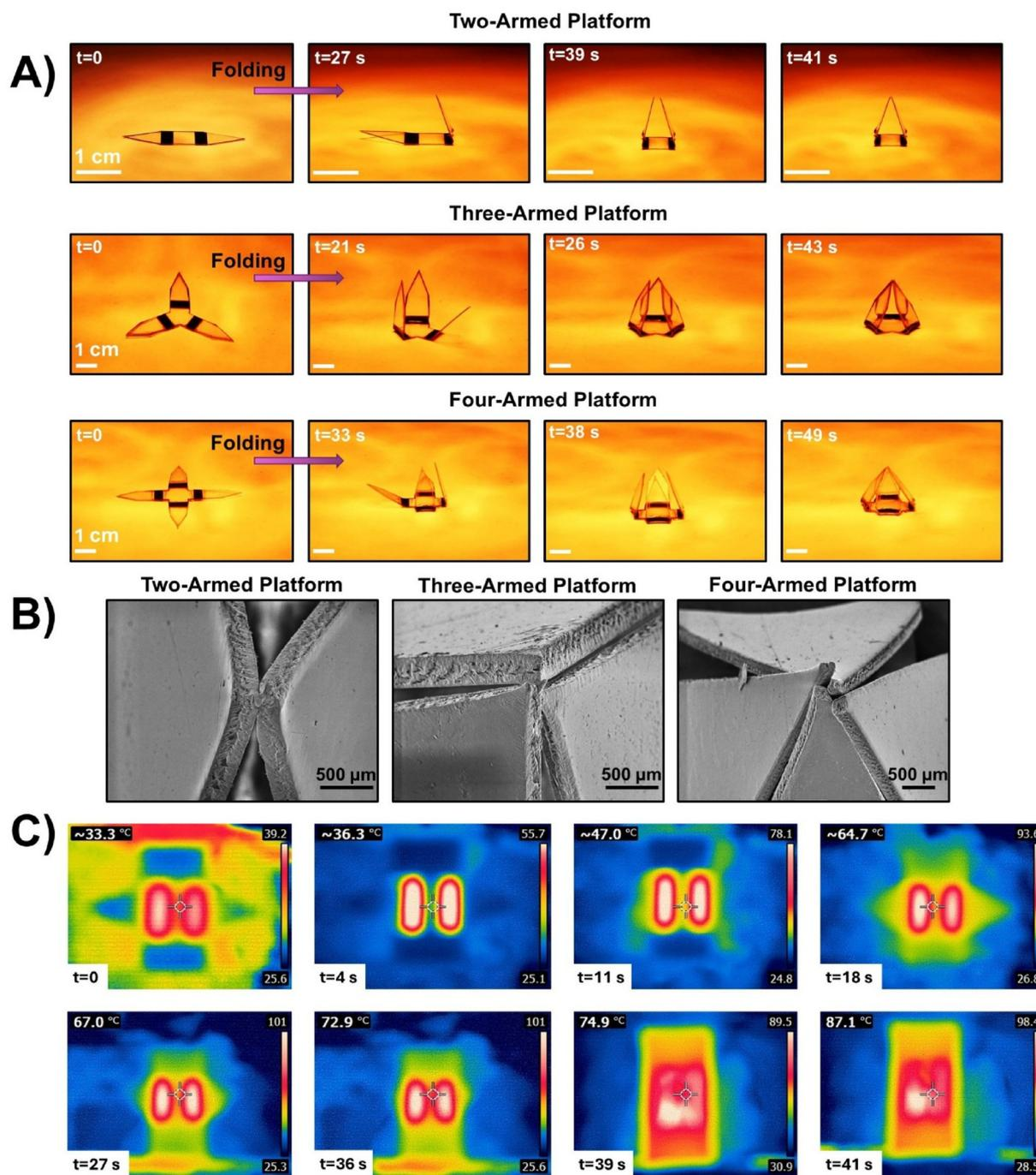
**Fig. 2** Snapshot images of the 2-, 3-, and 4-armed PS platforms folding under IR light illumination (250 W) (A). SEM images of the folded 2-, 3-, and 4-armed PS platforms (B). Thermal camera images of the folding process of a 2-armed PS platform with time (C).
