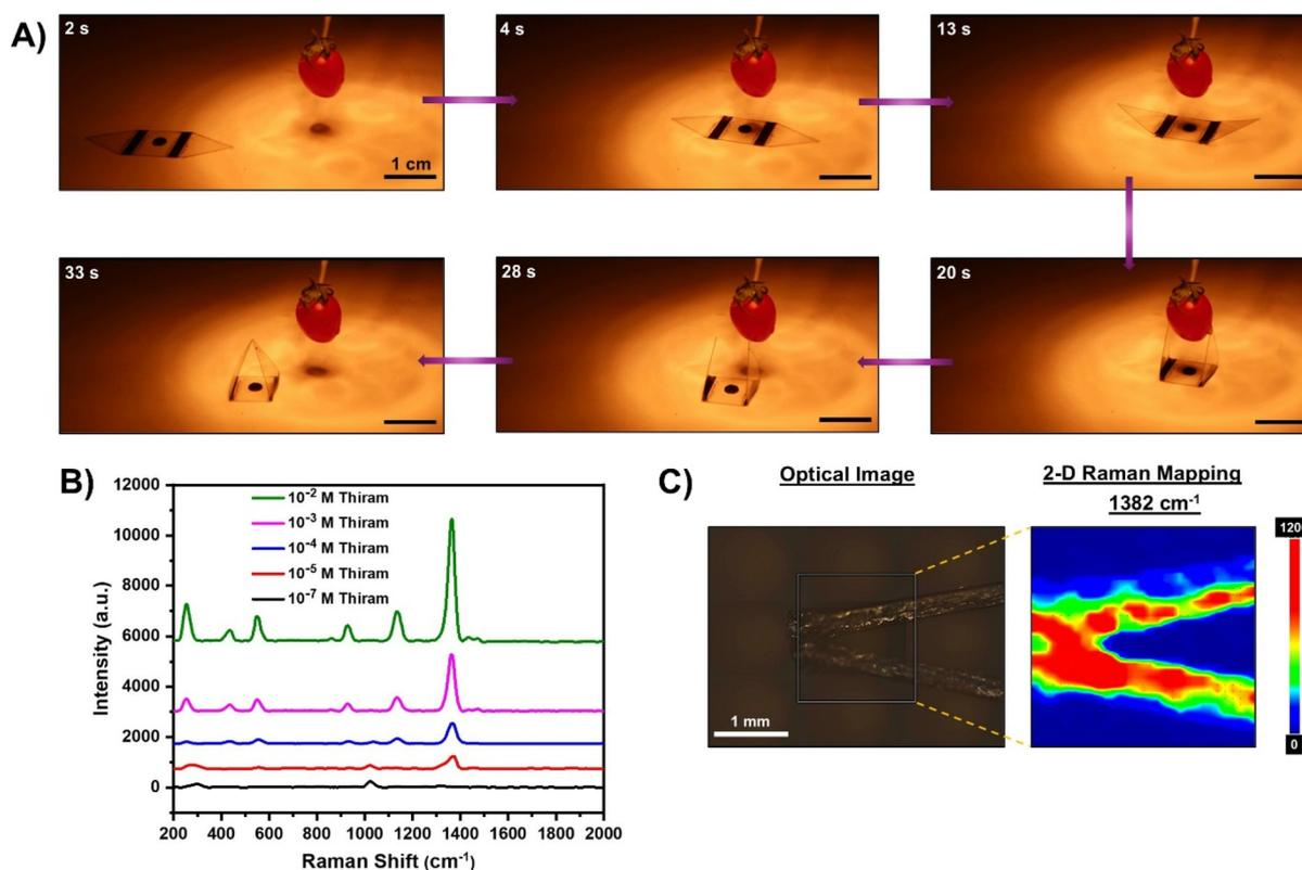
**Fig. 7** (A) Snapshot images of sample collection from Thiram-impregnated cherry tomato using two-armed polymeric platforms. (B) SERS spectra of Thiram with different concentrations collected from a target using two-armed PS platforms. (C) 2D SERS Raman mappings of the collected Thiram molecules on the platforms for the  $1382\text{ cm}^{-1}$ .
