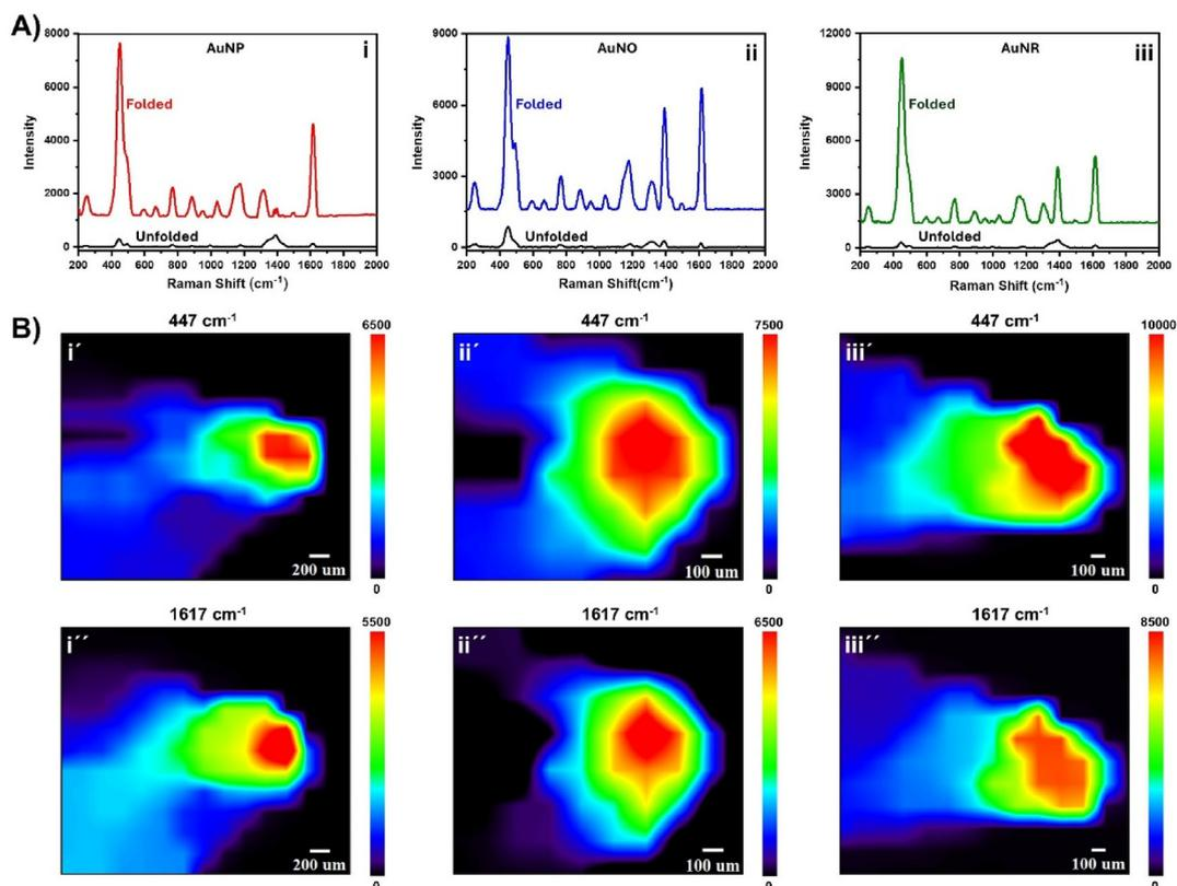
**Fig. 4** SERS spectra of MB collected from AuNP- (i), AuNO-, and AuNR-(iii) decorated 2-armed PS platforms before and after folding (A). 2D SERS Raman mapping of the folded AuNP- (i' and i''), AuNO- (ii' and ii''), and AuNR-(iii' and iii'') decorated 2-armed PS platforms for the 447 and 1617  $\text{cm}^{-1}$  peaks of MB (B).
