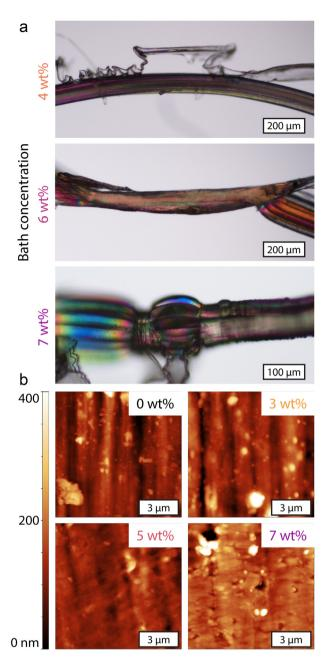
Fig. 4 (a) POM images of 4 wt%, 6 wt%, and 7 wt% bath concentrations demonstrating adherence of the CS coating to the fiber. (b) Representative 10  $\times$  10  $\mu$ m<sup>2</sup> AFM topography images (z-scale: 400 nm) for 0 wt%, 3 wt%, 5 wt%, and 7 wt% bath concentrations.
