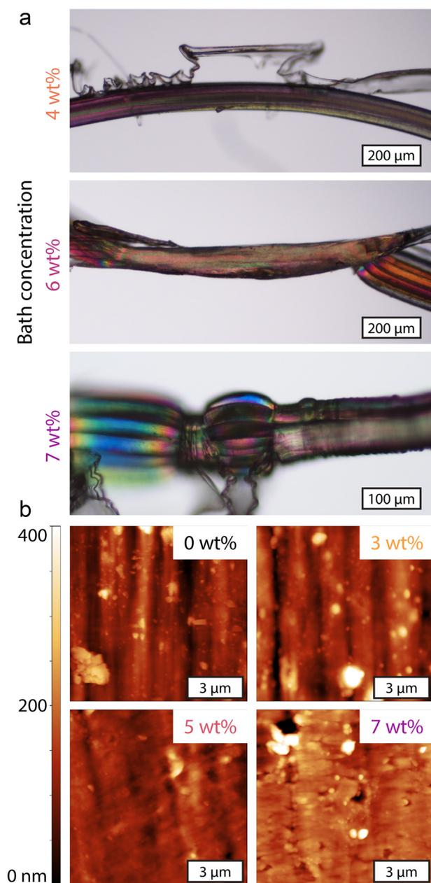
**Fig. 4** (a) POM images of 4 wt%, 6 wt%, and 7 wt% bath concentrations demonstrating adherence of the CS coating to the fiber. (b) Representative  $10 \times 10 \mu\text{m}^2$  AFM topography images (z-scale: 400 nm) for 0 wt%, 3 wt%, 5 wt%, and 7 wt% bath concentrations.
