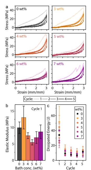
Fig. 3 (a) Stress-strain diagrams from cyclic tensile testing of the CScoated elastane fibers at different CS concentrations (0 wt%, 3 wt%, 4 wt%, 5 wt%, 6 wt%, and 7 wt%) performed for 5 hysteresis cycles. (b) Results of the elastic modulus determined from the first cycle for the different CS concentrations. (c) Dissipated energy obtained for each cycle for the different CS concentrations by calculating area under the hysteresis curves.
