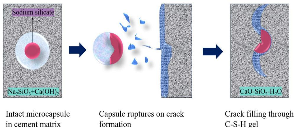
**Fig. 12** Mechanism of crack healing by sodium silicate microcapsules in cement matrix.
