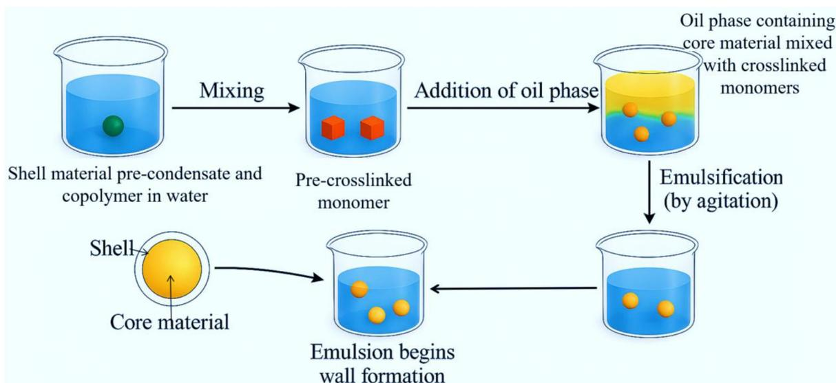
Fig. 5 Schematic representation of the *in situ* polymerization process showing stepwise encapsulation and shell formation around the core material, forming microcapsules sized 10–500  $\mu\text{m}$ .
