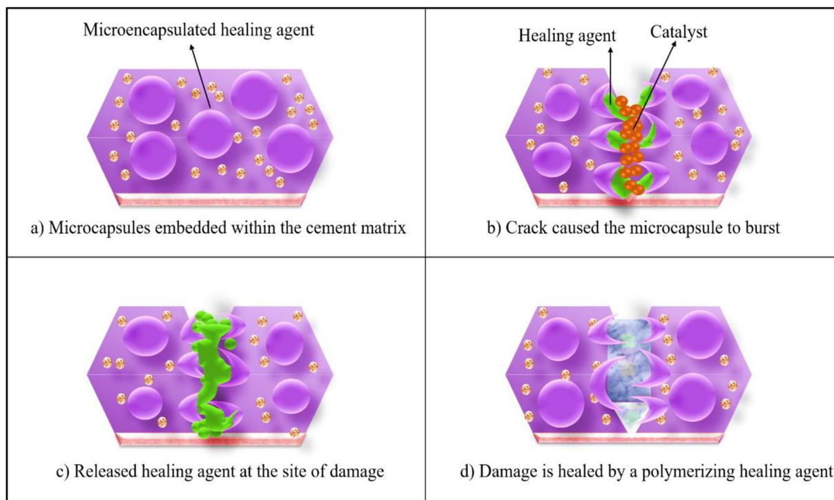
**Fig. 4** Schematic illustration of autonomic self-healing *via* microencapsulation, demonstrating the rupture of capsules (capsule size in  $\mu\text{m}$ ) and release of healing agents upon crack formation.
