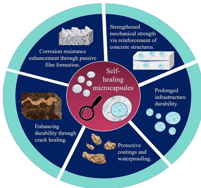
Fig. 11 Application of microcapsules in CBMs.
