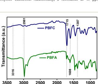
Fig. 1 FT-IR spectra of PBFC and PBFA.
