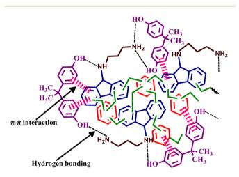
Scheme 3 Schematic representation of BPA adsorption mechanism on PBFA.
