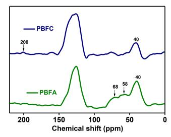
Fig. 2 Solid state <sup>13</sup>C NMR spectra of PBFC and PBFA.
