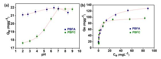
Fig. 6 (a) Effect of pH and (b) effect of initial concentration of BPA adsorption onto PBFC and PBFA at 298 K (20 mg adsorbent, 25 mL of 20 mg L<sup>-1</sup> BPA).
