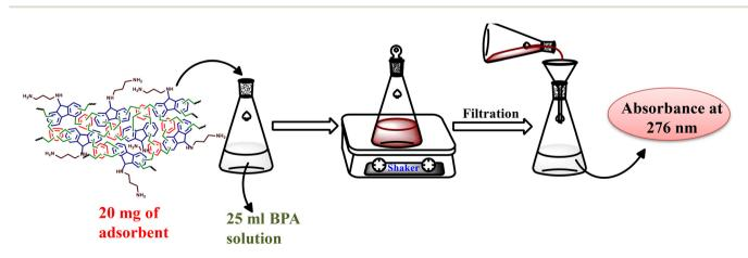
Scheme 2 Procedure for the adsorption experiment.
