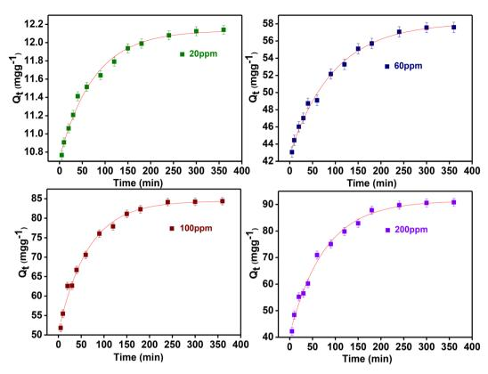
Fig. 7 Effect of contact time on adsorption at various concentrations of BPA solution (20 mg adsorbent, 25 mL BPA solution, 298 K).
