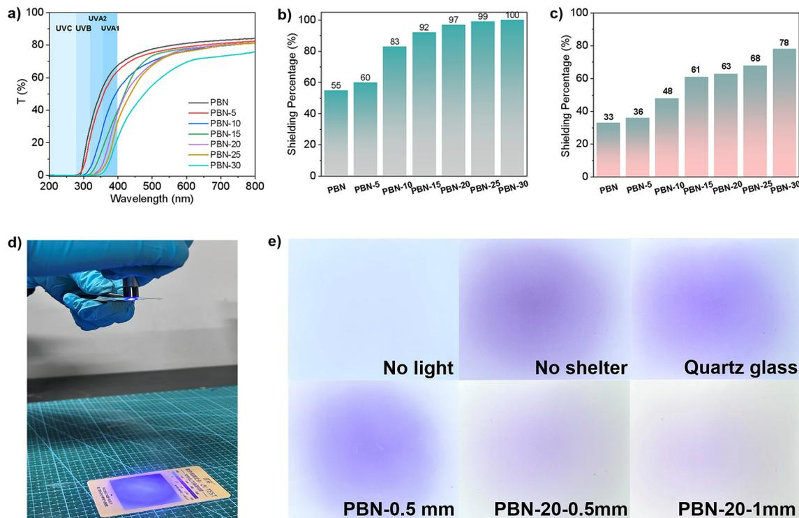
**Fig. 6** (a) Ultraviolet transmission spectra of a series of PBN and PBN-MDE films (thickness of 0.5 mm). (b) Shielding percentage at 340 nm for PBN and PBN-MDE films. (c) Shielding percentage at 400 nm for PBN and PBN-MDE films. (d) Experimental demonstration of the UV light beam irradiating the UV test card. (e) Photos of the UV light beam irradiating the UV test card under different conditions.
