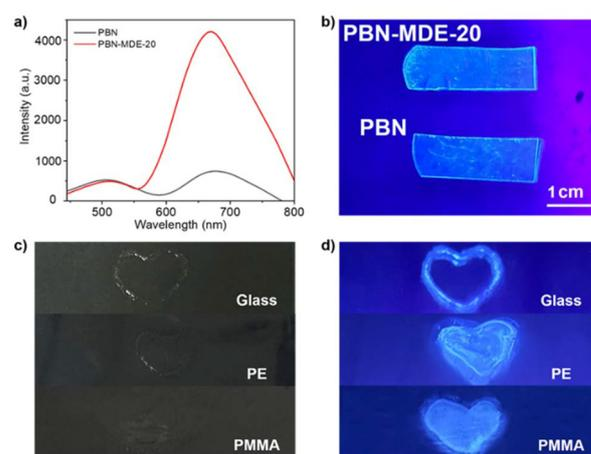
**Fig. 5** Fluorescence properties. (a) Fluorescence spectra of the films of PBN and PBN-MDE-20 with light excitation at 270 nm (thickness, 0.2 mm). (b) Comparison of fluorescence images of PBN and PBN-MDE-20 film excited by UV light of 365 nm. Digital images of heart-shaped patterns in different materials, exposed to natural light (c) and UV light of 365 nm (d).
