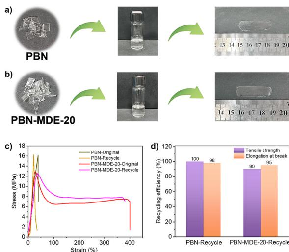
**Fig. 4** Recycling properties of PBN and PBN-MDE-20 polymer. (a) and (b) Recycling study. The PBN (a) and PBN-MDE-20 (b) films were cut and dissolved in DCM, and the recovered films were obtained by drying the organic solvent. (c) Stress-strain curves of PBN and PBN-MDE-20 before and after recovery. (d) The bar graph of recovery efficiency of PBN and PBN-MDE-20 films.
