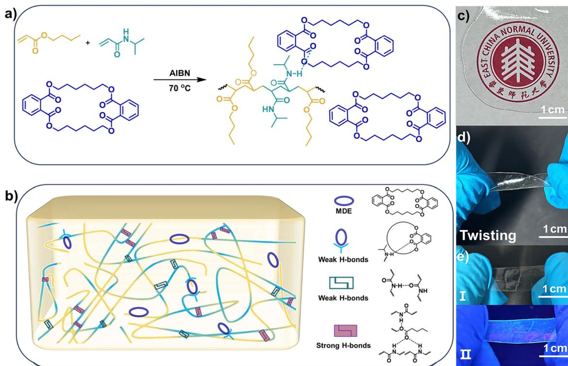
**Scheme 1** Synthesis of scorpion-inspired fluorescent polymers PBN-MDE. (a) Synthesis of self-healing PBN-MDE elastomers. (b) Schematic illustration of the polymer structure in PBN-MDE. Optical images of (c) light transmittance, (d) flexibility, and (e) fluorescence under UV light of PBN-MDE.
