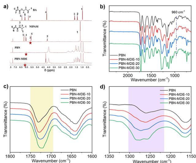
**Fig. 1** Structural characterizations of PBN and PBN-MDE. (a) <sup>1</sup>H NMR and (b), (c), and (d) FT-IR spectra at room temperature.
