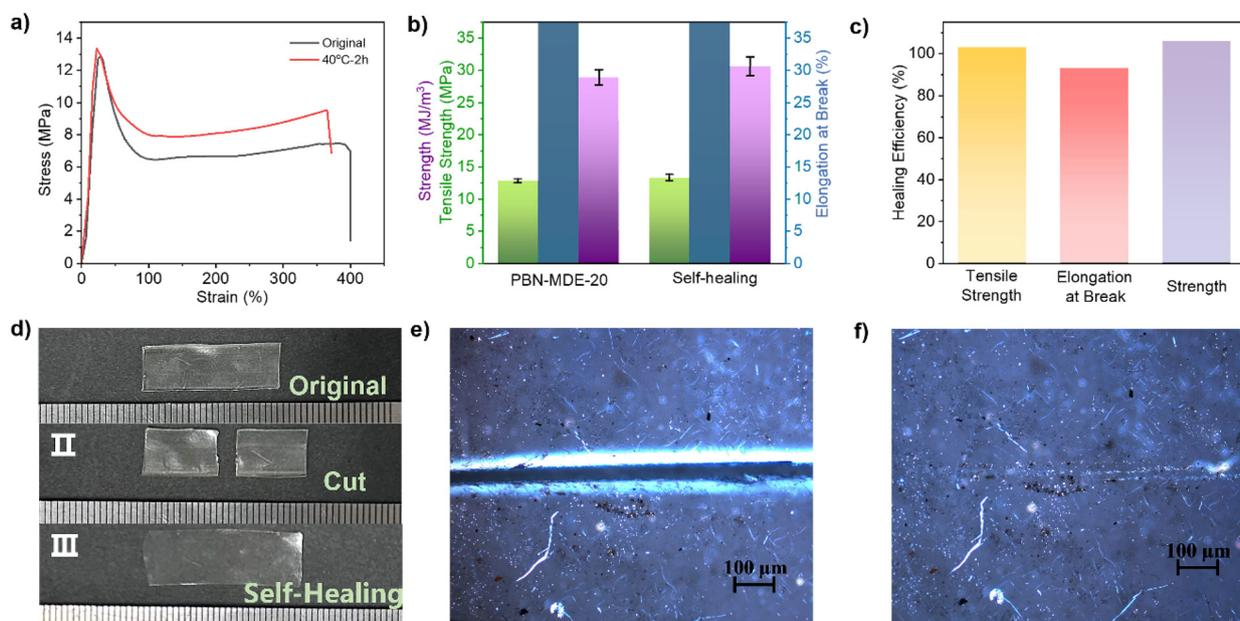
**Fig. 3** Self-healing behavior of PBN-MDE-20. (a) Stress–strain curves before and after self-healing. (b) The bar graph of toughness, tensile strength, and elongation break. (c) The bar graph of self-healing efficiency. (d) Images of the surface-damaged sample and healed sample at 40 °C. (e and f) Optical microscope images of the damaged state (e) of film and the healed state (f) after 2 h (scale bar: 100 μm).
