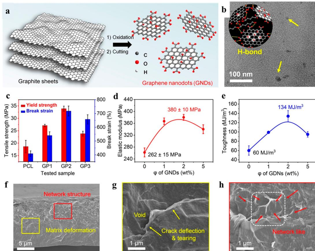
**Fig. 10** (a) Diagram showing the synthesis of GOD, (b) the cross-sectional transmission electron microscopy (TEM) image of a PCL/GOD nanocomposite, (c) tensile strength and breaking strain, (d) elastic modulus, and (e) tensile toughness for poly( $\epsilon$ -caprolactone) (PCL) and PCL/graphene nanodots (GNDs). (f–h) SEM photographs displaying the fracture morphology of PCL with 2 wt% GNDs. (a–h) Reproduced with permission.<sup>88</sup> © 2023 American Chemical Society.
