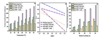
Fig. 7 (a) Proton conductivity ( $\sigma$ ) as a function of temperature at 95% RH, (b) logarithmic plot of proton conductivity vs. 1000/T, and (c) proton conductivity at different relative humidities at 65 °C of the prepared SSC-PFSA and composite membranes.
