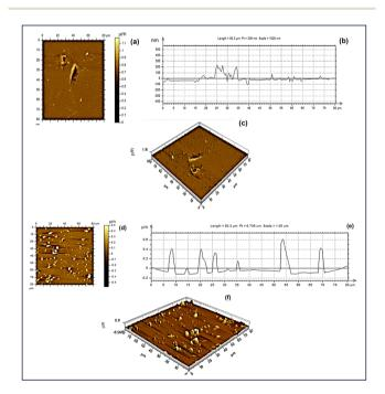
**Fig. 4** AFM images of (a–c) pristine SSC-PFSA and (d–f) Aq-PABS-f-SWCNT-0.5 wt% composite membranes.
