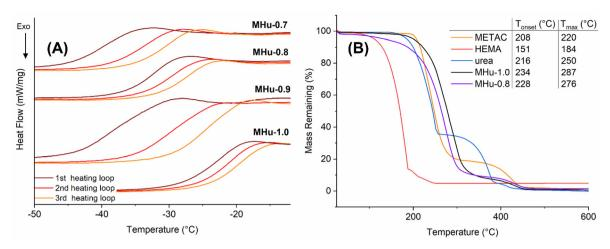
Fig. 5 (A) DSC thermograms of eutectic mixtures heated from -60 to 70 °C (first heating loop excluded). Thermograms from different samples have been offset for clarity. (B) TGA traces of eutectic components compared to the binary mixture, MHu-1.0 and the ternary mixture MHu-0.8, with onset and max rate temperatures tabulated.
