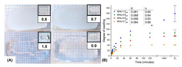
Fig. 7 (A) Photos of eutectogels at  $S_{eq}$  with their size as cured shown in insets. Light blue grid lines are  $5 \times 5$  mm. (B) Swelling kinetics and swelling ratios. Error bars for eutectogels at equilibrium swelling represent standard deviation, n = 3. Inset text shows fit parameters for the Korsmeyer-Peppas mass transfer model for gel swelling.
