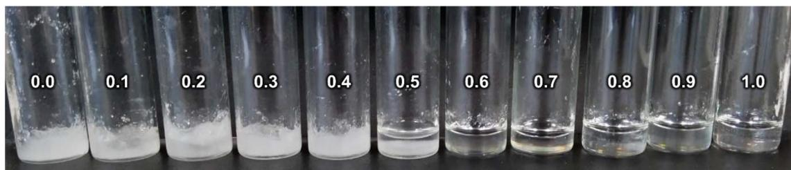
Fig. 2 Photo of MHu-*x* PE mixtures with molar ratios of  $x:(1-x):2$ , where *x* represents the METAC fraction of the monomers as listed for each vial in the image.
