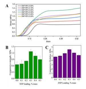
Fig. 7 Mechanical properties of rigid polyurethane foam (RPUF) with varying addition of silica nano-particles (SNP): (A) Compressive stress–strain curve. (B) compressive strength, and (C) compressive modulus.
