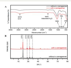
Fig. 2 (A) Fourier transform infrared spectroscopy (FTIR) and (B) X-ray diffraction (XRD) spectra of synthesized silica nanoparticles (SNP) of both with and without κ-carrageenan.
