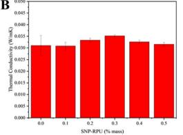
Fig. 8 (A) Thermogravimetric analysis (TGA) and (B) thermal conductivity of rigid polyurethane foam (RPUF) at varying addition of silica nanoparticles (SNP).
