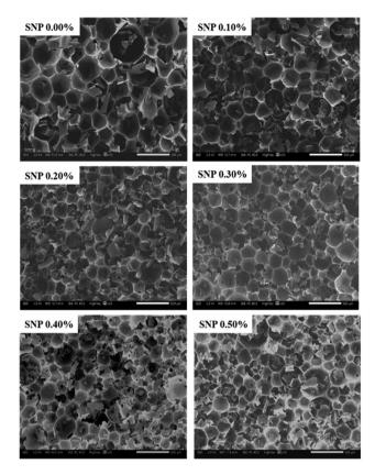
Fig. 6 Scanning electron microscope (SEM) micrographs (50x magnification) of rigid polyurethane foam (RPUF) foams at varying additions of silica nanoparticles (SNP).
