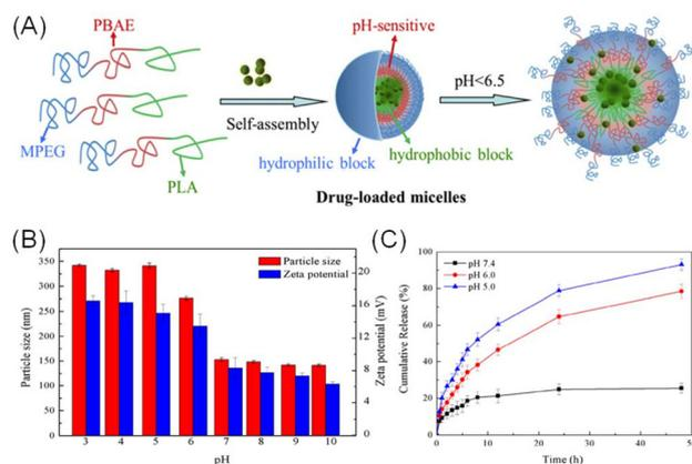
**Fig. 2** (A) Schematic illustration of pH-sensitive drug-loaded micelles formed by MPEG-*b*-PBAE-*b*-PLA copolymers. (B) Particle size and zeta potential of micelles at different pH values. (C) Cumulative drug release at pH 7.4, 6, and 5. Adapted with permission ref. 130. Copyright 2018 Elsevier.
