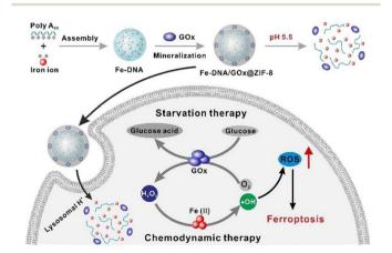
Fig. 3 The MOF nanoparticles formed assembly *via* the coordination of DNA and metal Fe<sup>2+</sup> ions. Adapted with permission ref. 133. Copyright 2021 Elsevier
