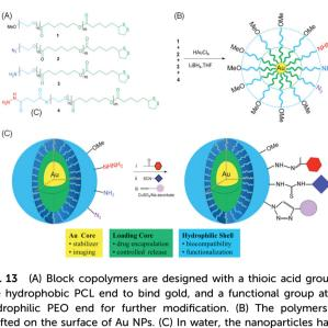
Fig. 13 (A) Block copolymers are designed with a thioic acid group at the hydrophobic PCL end to bind gold, and a functional group at the hydrophilic PEO end for further modification. (B) The polymers are grafted on the surface of Au NPs. (C) In water, the nanoparticles have a gold core (yellow); a hydrophobic PCL layer (green) for loading hydrophobic drugs; and a biocompatible PEO shell (blue). Adapted with permission ref. 213. Copyright 2011 American Chemical Society.
