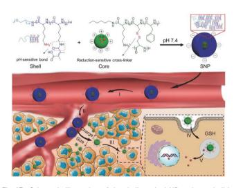
Fig. 17 Schematic illustration of the shell-stacked NPs, whose shell is formed via electrostatic interaction of dimethylmaleic anhydridemodified polypeptide (shell-DMMA), enabling sharp size reduction (from 145 nm to 40 nm) and charge reversal (from -7.4 mV to 8.2 mV) in the acidic tumour microenvironment. Adapted with permission ref. 290. Copyright 2017 John Wiley & Sons.
