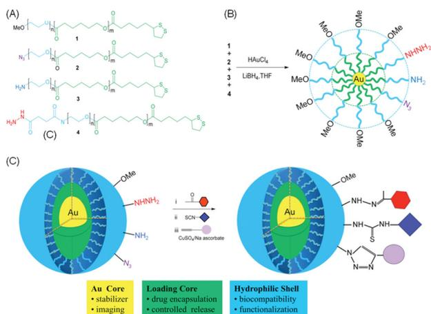
**Fig. 13** (A) Block copolymers are designed with a thioic acid group at the hydrophobic PCL end to bind gold, and a functional group at the hydrophilic PEO end for further modification. (B) The polymers are grafted on the surface of Au NPs. (C) In water, the nanoparticles have a gold core (yellow); a hydrophobic PCL layer (green) for loading hydrophobic drugs; and a biocompatible PEO shell (blue). Adapted with permission ref. 213. Copyright 2011 American Chemical Society.
