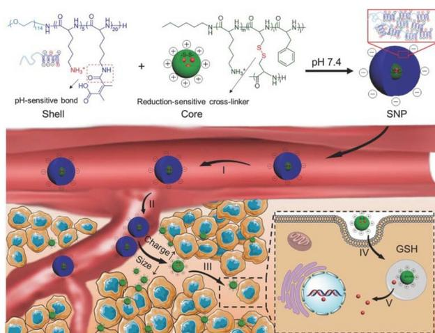
**Fig. 17** Schematic illustration of the shell-stacked NPs, whose shell is formed *via* electrostatic interaction of dimethylmaleic anhydride-modified polypeptide (shell-DMMA), enabling sharp size reduction (from 145 nm to 40 nm) and charge reversal (from  $-7.4$  mV to  $8.2$  mV) in the acidic tumour microenvironment. Adapted with permission ref. 290. Copyright 2017 John Wiley & Sons.
