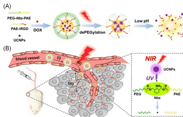
**Fig. 20** (A) Schematic illustration of pH-sensitive NPs composed of PEG-Nbz-PAE-Nbz-PEG (HTMP) and iRGD-PAE-iRGD (iPHT) polymers, with UCNPs used for NIR-to-UV conversion, triggering cleavage of the Nbz linkers and dePEGylation, which (B) then activates iRGD for enhanced tumour penetration and drug release. Adapted with permission ref. 304. Copyright 2019 American Chemical Society.
