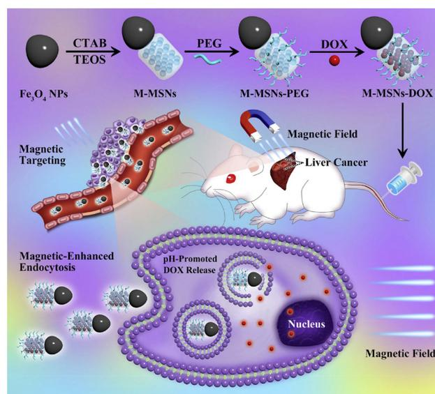
**Fig. 15** Schematic illustration of Janus “nano-bullet” multifunctional NPs (M-MSNs-DOX) integrate a magnetic Fe<sub>3</sub>O<sub>4</sub> head and a DOX-loaded mesoporous SiO<sub>2</sub> body, enabling magnetically enhanced endocytosis and pH-responsive drug release. Adapted with permission ref. 230. Copyright 2016 Elsevier.
