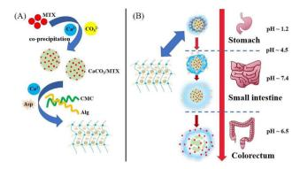
Fig. 6 (A) Schematic illustration of the preparation of methotrexate (MTX)-loaded calcium carbonate ( $CaCO_3$ ) nanoparticles. (B) The nanocomposite particles remain stable in the acidic gastric environment (pH  $\sim$ 1.2), begin to swell and release MTX in the small intestine (pH  $\sim$ 7.4), and ultimately achieve targeted drug release in the colorectum (pH  $\sim$ 6.5). Adapted with permission ref. 151. Copyright 2021 Elsevier.
