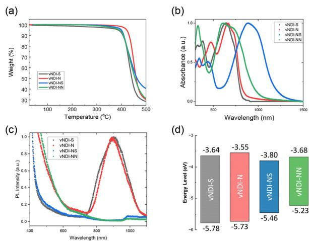
**Fig. 2** (a) TGA thermograms, (b) UV-vis-NIR film absorption spectra, (c) photoluminescence (PL) emission spectra, and (d) energy levels (obtained) by cyclic voltammetry (CV) of vNDI-based polymer films.
