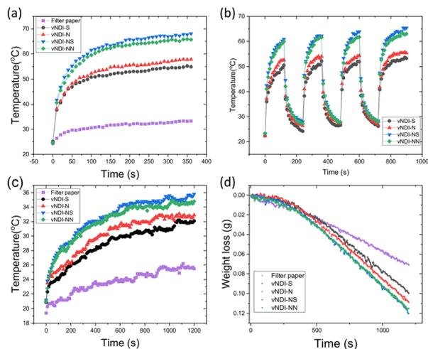
**Fig. 6** Temperature changes in (a) dry and (c) wet photothermal membranes with **vNDI**-based polymers and filter paper (control sample) under simulated sunlight irradiation for 6 minutes. (b) The repeated simulated sunlight irradiation at intervals of 2 minutes. (d) The weight loss of wet photothermal membranes with **vNDI**-based polymers under simulated sunlight irradiation for 20 minutes.
