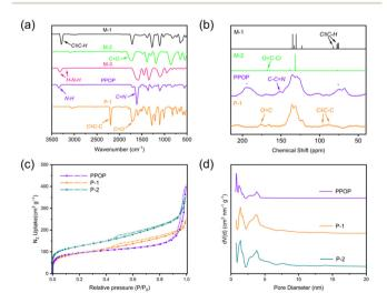
Fig. 1 (a) FT-IR spectroscopy of M-1 to M-3, PPOP, and P-1; (b) 13C NMR spectra of M-1 to M-2 in solutions, and PPOP and P-1 in the solid state; (c) nitrogen adsorption and desorption isotherm of PPOP, P-1, and P-2; and (d) pore size distribution curve of PPOP, P-1 and P-2. Asterisks denote the spinning sidebands.
