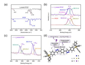
Fig. 5 (a) FT-IR spectra of pristine and iodine-loaded PPOP; (b) N 1s XPS spectra for pristine and iodine-loaded PPOP; (c) XPS spectra of I 3d for  $I_2$ -loaded PPOP; and (d) schematic representation of the iodine adsorption mechanism by PPOP.
