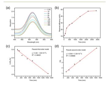
Fig. 3 (a) UV-vis adsorption spectra of the iodine solutions after being treated with **PPOP** at different time intervals; (b) effect of adsorption time on the adsorbed amount of iodine by **PPOP** suspension in n-hexane (1 mg mL $^{-1}$ ); (c) the pseudo-first-order model; and (d) the pseudo-second-order model.
