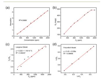
Fig. 4 (a) The fitting of the absorption value vs. concentration of  $l_2$  in n-hexane solution with a relatively good linearity. (b) Effect of the initial iodine concentrations on the adsorption amount of iodine by PPOP suspension in n-hexane (1 mg mL $^{-1}$ ); (c) the Langmuir model; and (d) the Freundlich model.
