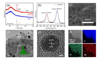
**Fig. 6** (a) XRD patterns of **PPOP** and PPOP-Ag; (b) Ag 3d XPS spectra of PPOP-Ag; (c) SEM image of PPOP-Ag; (d) TEM image of PPOP-Ag (inset: histogram illustrating the particle size distribution); (e) HRTEM image of PPOP-Ag; and (f) SEM image and energy-dispersive X-ray spectroscopy elemental mappings of PPOP-Ag.
