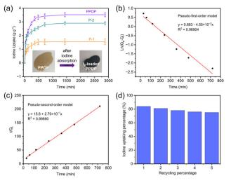
Fig. 2 (a) Gravimetric  $I_2$  uptake of PPOP, P-1, and P-2 as a function of time at 75 °C (inset: color changes of PPOP after absorbed iodine); (b) pseudo-first-order model spectra of PPOP; (c) pseudo-second-order model spectra of PPOP; and (d) recyclability of PPOP for iodine capture.
