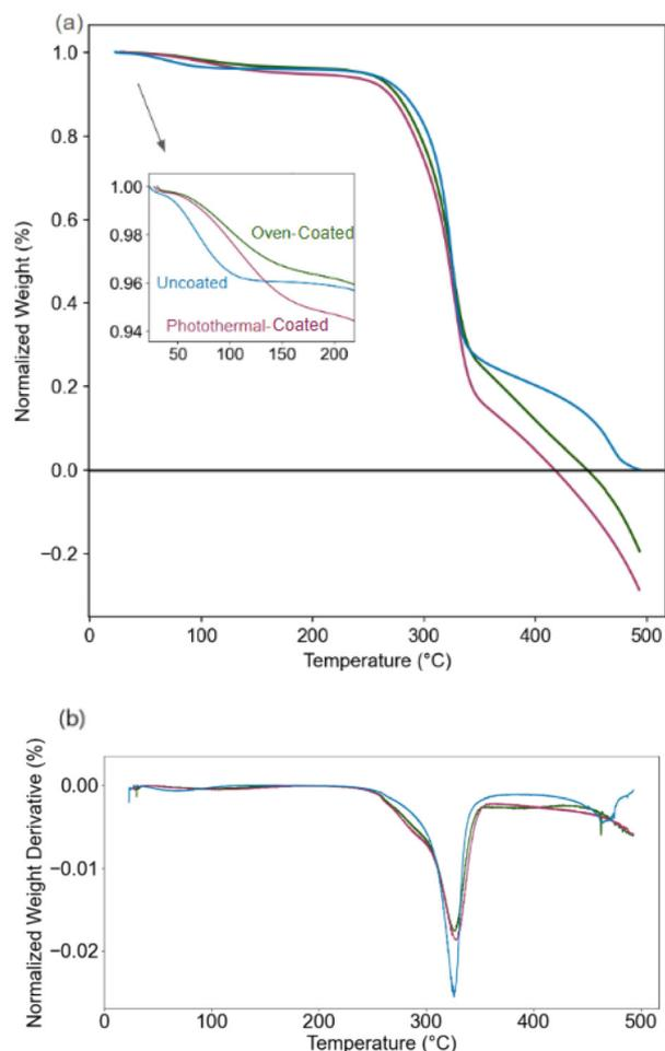
**Fig. 4** Results of TGA measurements on uncoated (blue), oven-coated (green), and photothermal-coated (dark magenta) samples. (a) TGA traces for each sample, normalized to the amount of paper present. The uncoated sample (blue) is considered 100% paper. The inset focuses on the region below 200 °C. (b) Derivative plot of the traces shown in (a).
