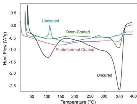
**Fig. 3** DSC data for photothermal-coated (dark magenta), oven-coated (green), uncoated (blue), and uncured (black) paper samples. All curves were normalized to the mass of the paper present in the sample.
