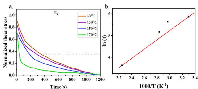
Fig. 7 (a) Normalised stress relaxation plots of the dual dynamic vitrimer. (b) Arrhenius plot of  $\ln(\tau)$  versus  $1000/T$  of E<sub>1</sub>.
