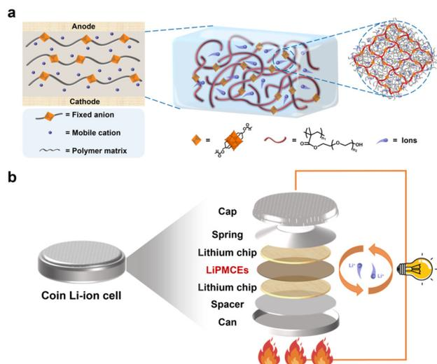
**Fig. 1** (a) Schematic of the microstructure of the PMCEs, and counter-cation transfer mechanism by side chains. (b) Schematic of the 0.16% LiPMCEs assembled into a coin cell structure that can be used under high-temperature conditions.
