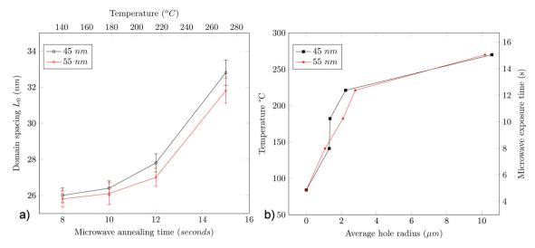
Fig. 6 (a) TA  $L_0$  that is 26 nm increases substantially for both h = 45 nm and h = 55 nm PS-b-PMMA films by increasing the microwave annealing time from 8 s to 15 s. See the text for discussion. The corresponding temperatures of the microwave annealing time for 8 s, 10 s, 12 s, and 15 s are respectively 141 °C, 182 °C, 221 °C, and 270 °C. (b) The average hole radius at 8 s of microwave annealing continuously increases with the increment of the microwave annealing time up to 15 s.
