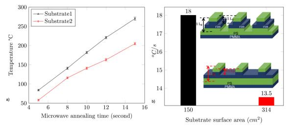
Fig. 7 (a) Temperature of the BCP thin film's substrate, high-resistivity B-doped silicon wafer, P-type2, named Substrate1 and Substrate2 is recorded starting from 5 s until 15 s. (b) Substrate1, which has an area of 150 cm<sup>2</sup> and Substrate2 having 314 cm<sup>2</sup> showed average temperature gradients of 18 °C s<sup>-1</sup> and 13.5 °C s<sup>-1</sup>, respectively.
