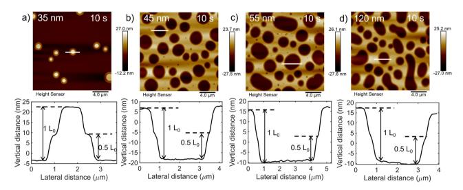
Fig. 5 BCP thin films with thicknesses of 10 s microwave annealed of (a) 35 nm, (b) 45 nm, (c) 55 nm, and (d) 120 nm; island-on-island terrace formation of concentric  $0.5L_0$  islands at 35 nm *versus* concentric  $0.5L_0$  holes: 45 nm, 55 nm, and 120 nm, respectively.
