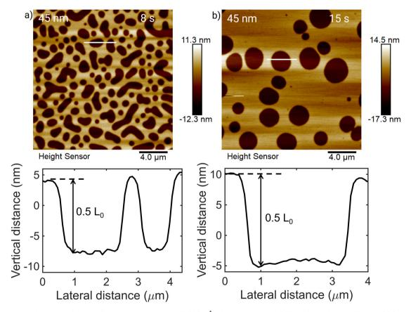
Fig. 8 Surface morphology on Substrate2, with a heating rate of 13.5 °C s<sup>-1</sup>, which created only 0.5L<sub>0</sub> without rims for 45 nm in (a) 8 s and (b)15 s.
