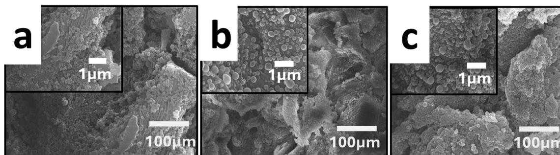
Fig. 5 SEM images of PA1 (a), PA2 (b), and PA3 (c) after adsorption of (+)PVC NPs from the solution.
