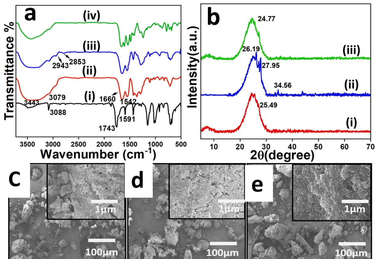
**Fig. 1** FTIR spectra (a, i–iv) and XRD patterns (b, i–iii) of as-synthesised PA1 (—), PA2 (—), and PA3 (—). The FTIR spectrum (a, i) of the starting material TMC is given for comparison. SEM micrographs of synthesised PA1 (c), PA2 (d), and PA3 (e). Similar micrographs for PA4, 5 and TA are given in the SI (Fig. S1).
