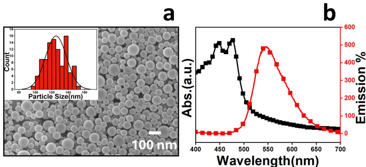
Fig. 2 SEM image of dry (a) and absorption and emission spectra (b) of water dispersion of (+)PVC NPs. The inset in (a) represents the size distribution of the particles calculated from SEM images. The SEM image of (–)PVC NPs is given in Fig. S3.
