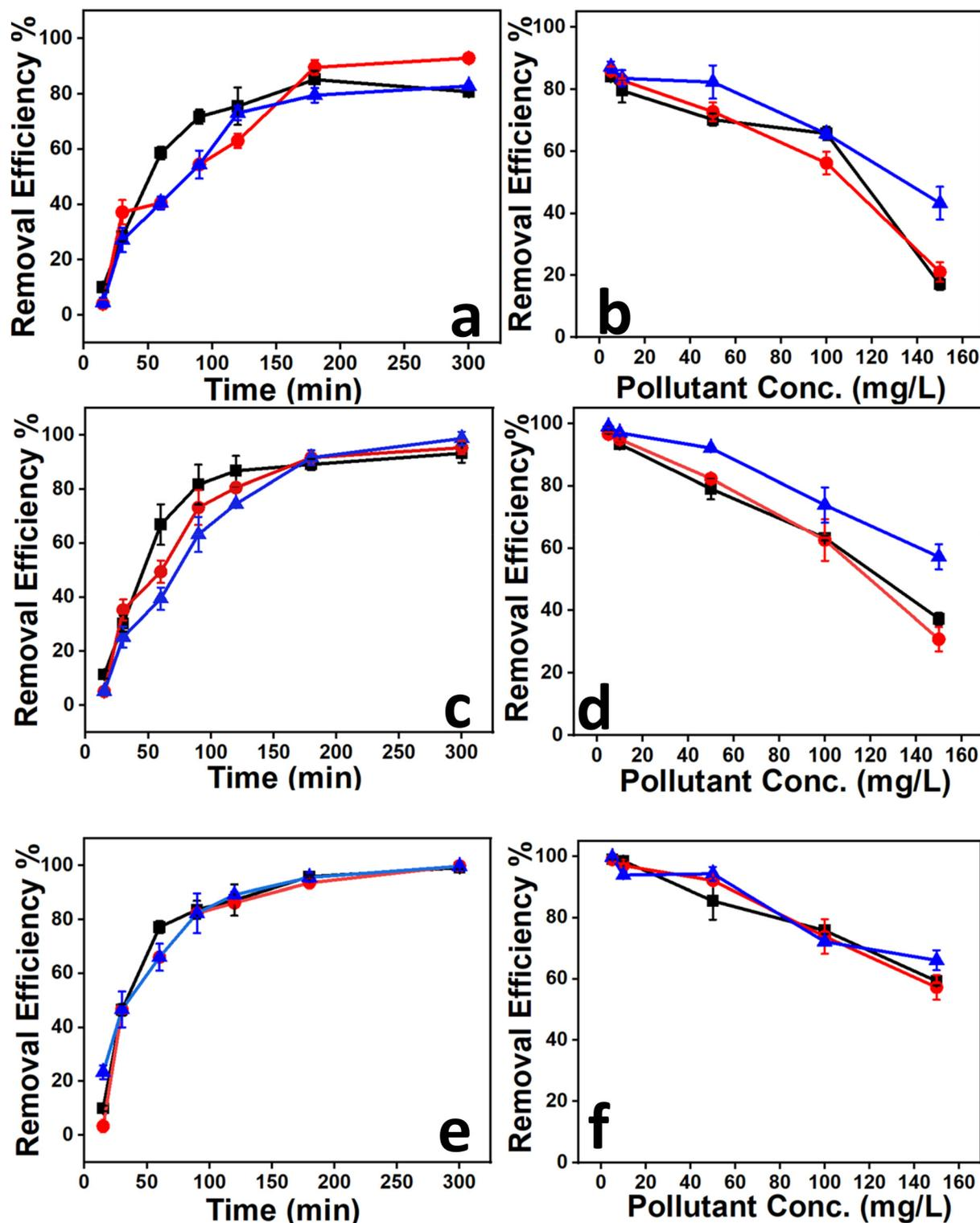
Fig. 4 Effect of time (0–300 min, a, c and e) and concentration (0–150 mg L<sup>-1</sup>, b, d and f) of -■- (+)PVC NPs, -●- -NR and -▲- -MB on removal efficiencies – PA1 (a and b), PA2 (c and d) and PA3 (e and f). The amount of all PAs used for the adsorption experiments was kept constant as 25 mg. For time dependent studies, the concentration of the pollutants was fixed at 50 mg L<sup>-1</sup>. The data for PA3, PA4, and TA are given in Fig. S6.
