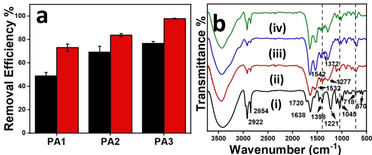
**Fig. 12** All PAs (25 mg) were tested for the removal of microplastic particles from the facial scrubber solution. The removal efficiencies (a) of PAs at different time points (■) 2 h and (■) 5 h, and FTIR spectra (b) of the facial scrubber (i) and the scrubber adsorbed on PA1 (ii), PA2 (iii) and PA3 (iv).
