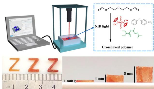
Fig. 6 RAFT stereolithography process under NIR light at 25 °C used to 3D print objects with different thicknesses. Reproduced with permission. Copyright 2021 American Chemical Society.<sup>85</sup>
