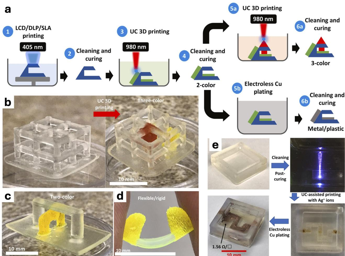
**Fig. 9** (a) Schematic representation of the proposed upconversion-assisted multimaterial stereolithography process. (b) Three-color print. (c) Two-color "bridge under another bridge". (d) Flexible/rigid print. (e) Processes for stereolithography printing metal/dielectric objects via upconversion-assisted crosslinking and selective metallization. Reproduced with permission. Copyright 2023 Elsevier.<sup>54</sup>
