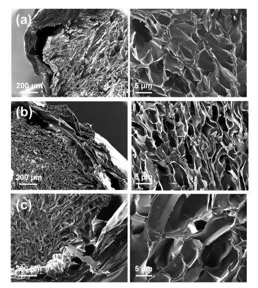
Fig. 5 Cross-section SEM images of (a) 50:50. (b) 70:30 and (c) 90:10 microtubular constructs filled with the clickHA hydrogel. Images showing the integration of the clickHA hydrogel and the PLA/PCL shell (left) and the honeycomb morphology of the clickHA hydrogel (right) are shown.
