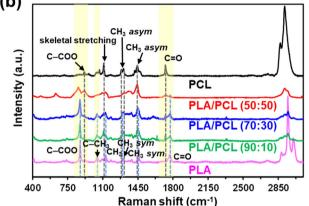
Fig. 2 (a) FTIR and (b) Raman spectra of films derived from neat PLA, 90:10 PLA/PCL, 70:30 PLA/PCL, 50:50 PLA/PCL and neat PCL.
