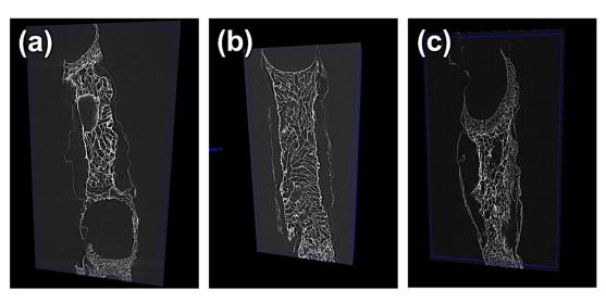
Fig. 6 μ-CT images of the clickHA hydrogels confined in (a) 50:50, (b) 70:30 and (c) 90:10 PLA/PCL tubular constructs.
