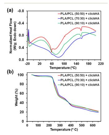
**Fig. 9** (a) DSC analyses (second heating scan) and (b) TGA thermograms of PLA/PCL microtubular constructs filled with the hydrogel.
