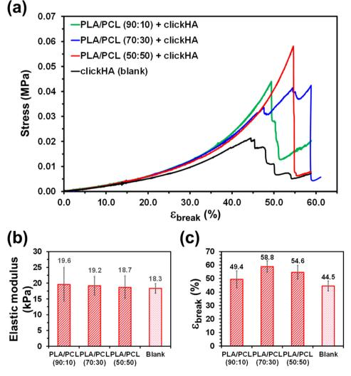
Fig. 8 (a) Representative uniaxial compressive curves for the clickHA hydrogel alone and clickHA-filled 90:10, 70:30 and 50:50 PLA/PCL microtubular constructs. Comparison of the (b) elastic modulus (E) and (c) elongation at break ( $\varepsilon_{\text{break}}$ ) values.
