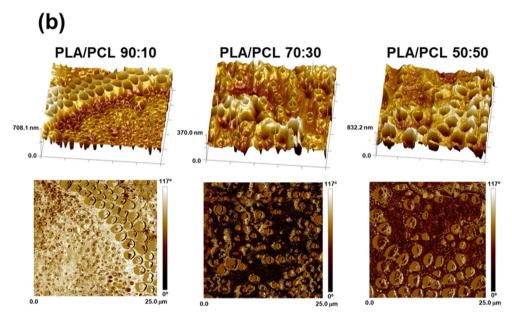
Fig. 1 (a) Scheme showing the process used to prepare self-standing PLA/PCL films of submicrometric thickness. (b) Representative topography (top) and phase (bottom) AFM images ( $25 \times 25 \mu m^2$ ) of PLA/PCL 90:10, 70:30 and 50:50 films.
