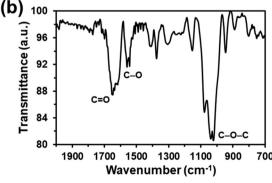
Fig. 4 (a) Variation in the gelation time against the [KOH]/[HA-SH] ratio. (b) FTIR spectrum of the clickHA hydrogel obtained after removing the 70:30 PLA/PCL tubular construct.
