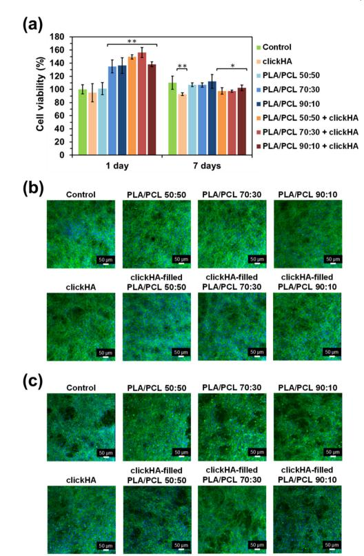
Fig. 10 (a) Cell viability assays for PLA/PCL blends, clickHA hydrogel and hydrogel-filled tubular constructs. (b, c) Confocal microscopy images of the different studied materials and constructs after (b) 1- and (c) 7-day cell incubation periods. Data are represented as mean ± standard deviation; n = 3 per group. Significance levels are as follows: \*p < 0.05, \*\*p < 0.01, determined by one-way ANOVA and Tukey's multiple comparisons test.
