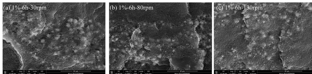
Fig. 8 The dispersion of tungsten powder in W/HDPE-v-1%-50 rpm-3 MPa-6 h composites from SEM graphs of cross-section: (a) 30 rpm; (b) 80 rpm; (c) 130 rpm.
