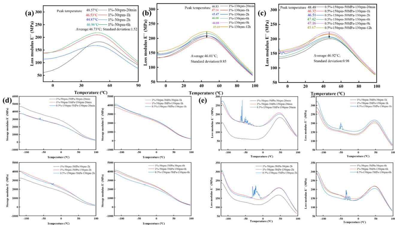
**Fig. 10** DMA graphs: the loss modulus of W/HDPE-v-1%-50 rpm-3 MPa-30 rpm-(20 min-6 h) (a); W/HDPE-v-1%-50 rpm-3 MPa-130 rpm-(20 min-12 h) (b); and W/HDPE-v-0.5%-150 rpm-5 MPa-130 rpm-(20 min-12 h) (c). Comparison of storage modulus among W/HDPE-v-1%-50 rpm-3 MPa-30 rpm, W/HDPE-v-1%-50 rpm-3 MPa-130 rpm, and W/HDPE-v-0.5%-150 rpm-5 MPa-130 rpm (d); comparison of loss modulus among W/HDPE-v-1%-50 rpm-3 MPa-30 rpm, W/HDPE-v-1%-50 rpm-3 MPa-130 rpm, and W/HDPE-v-0.5%-150 rpm-5 MPa-130 rpm (e).
