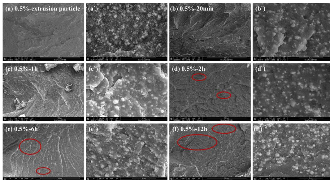
**Fig. 9** The cross-section morphology of W/HDPE-v-0.5%–150 rpm–5 MPa–130 rpm twin-screw particles (a–a') and hot-pressed samples with different thermal processing time: (b–b') 20 min, (c–c') 1 h, (d–d') 2 h, (e–e') 6 h, (f–f') 12 h.
