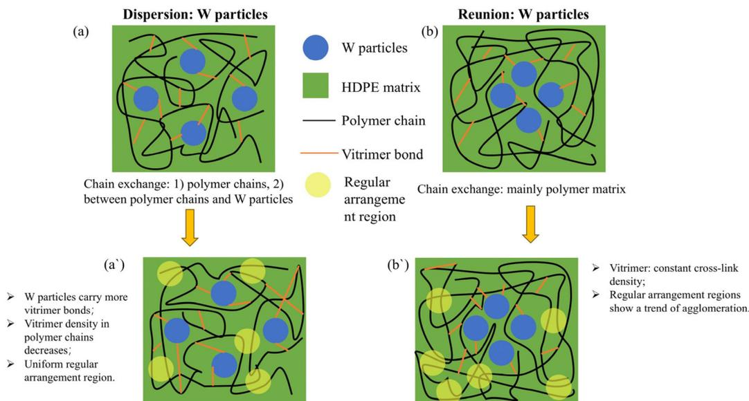
**Fig. 11** The schematic diagram of interfacial bonding, chain movement, and phase realignment in W/HDPE composites: (a and a') the situation of good W particle dispersion in the HDPE matrix; (b and b') the situation of worse W particle dispersion in the HDPE matrix.
