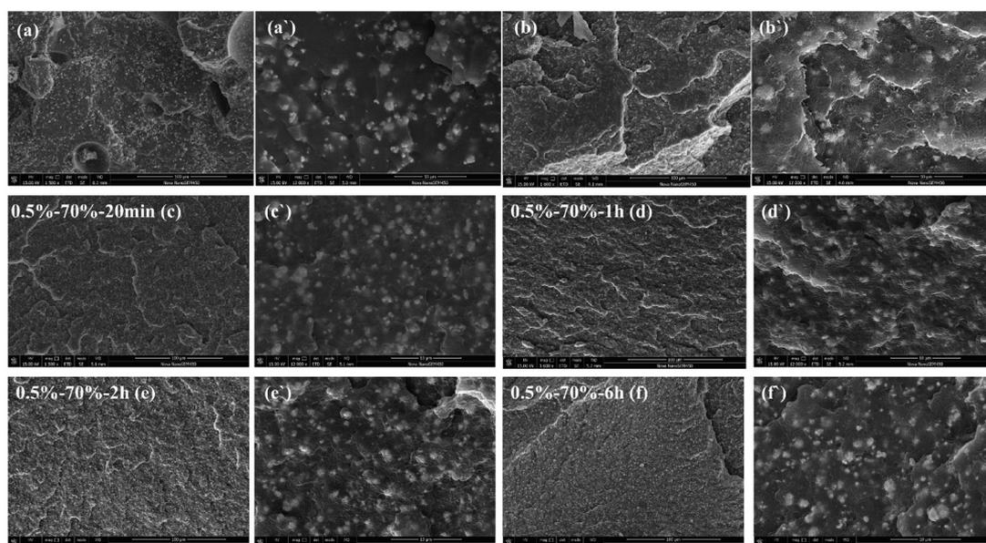
**Fig. 4** Dispersion of KH560-modified tungsten powder in an HDPE-v matrix: SEM graphs of cross-sections of samples (a and a') 70%W/PE composites with the addition of KH560 and POE-MA-modified agents; (b and b') HDPE-g-MA + W; (c and c') 70%W/HDPE-v-0.5%–100 rpm–6 MPa–200 rpm–20 min; (d and d') 70%W/HDPE-v-0.5%–100 rpm–6 MPa–200 rpm–1 h; (e and e') 70%W/HDPE-v-0.5%–100 rpm–6 MPa–200 rpm–2 h; (f and f') 70%W/HDPE-v-0.5%–100 rpm–6 MPa–200 rpm–6 h.
