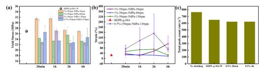
Fig. 12 The mechanical properties of each sample: (a) yield stress, (b) strain; gamma-ray shielding effects: HDPE-g-MA + W, W/HDPE-v-0.5%-150rpm-5 MPa-130 rpm-20 min, and W/HDPE-v-0.5%-150 rpm-5 MPa-130 rpm-6 h. (c) Comparison of gamma-ray shielding effects of each sample.
