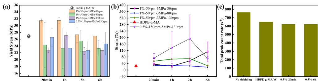
**Fig. 12** The mechanical properties of each sample: (a) yield stress, (b) strain; gamma-ray shielding effects: HDPE-g-MA + W, W/HDPE-v-0.5%–150 rpm–5 MPa–130 rpm–20 min, and W/HDPE-v-0.5%–150 rpm–5 MPa–130 rpm–6 h. (c) Comparison of gamma-ray shielding effects of each sample.
