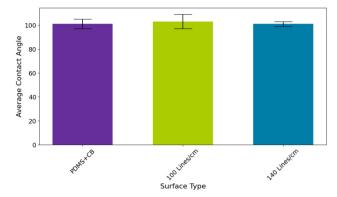
Fig. 7 Average contact angle measurements of water droplets on various nonpatterned and photothermally patterned surfaces.
