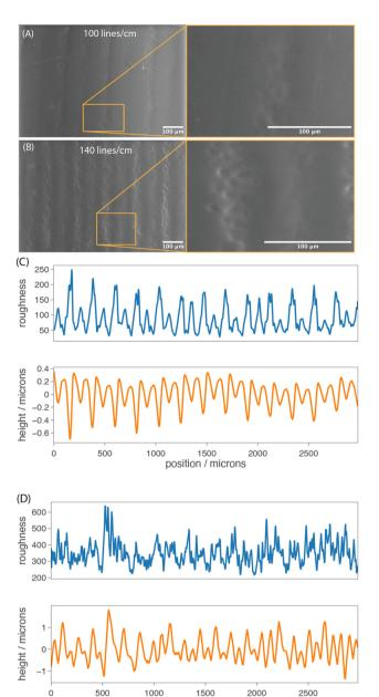
Fig. 5 SEM images of (A) 100 lines per cm and (B) 140 lines per cm surfaces as well as plots of roughness and average height for profiles running parallel to the lines for (C) 100 lines per cm and (D) 140 lines per cm samples.
