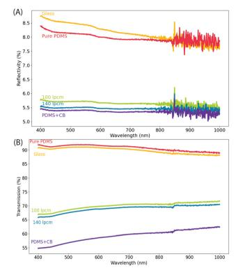
Fig. 6 (A) Reflectivity, and (B) transmission spectra of various surfaces compared to photothermally patterned PDMS.
