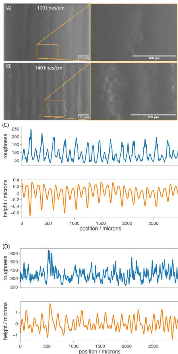
**Fig. 5** SEM images of (A) 100 lines per cm and (B) 140 lines per cm surfaces as well as plots of roughness and average height for profiles running parallel to the lines for (C) 100 lines per cm and (D) 140 lines per cm samples.
