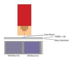
**Fig. 1** Schematic of photothermal patterning using a laser etcher. Control over the patterns can be done by changing the spacing between lines in a 'snake' pattern.
