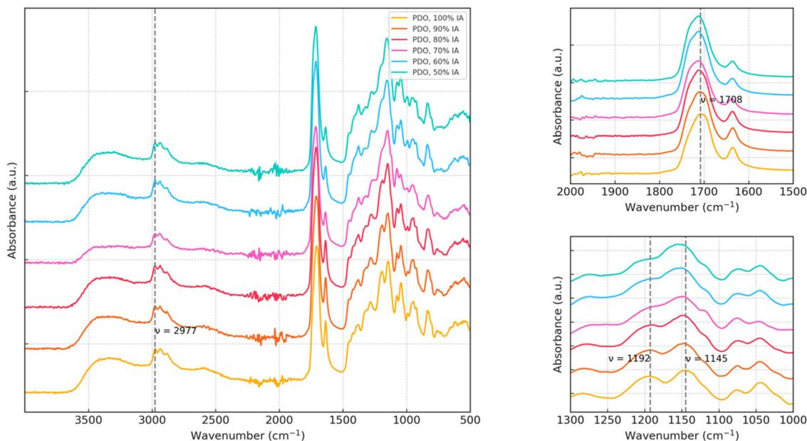
**Fig. 1** ATR-FTIR spectra of PDO oligoesters containing 50–100% itaconic acid with a balance of succinic acid. Inset plots for the wavenumber ranges of  $2000\text{--}1500 \text{ cm}^{-1}$  and  $1300\text{--}1000 \text{ cm}^{-1}$  are included.
