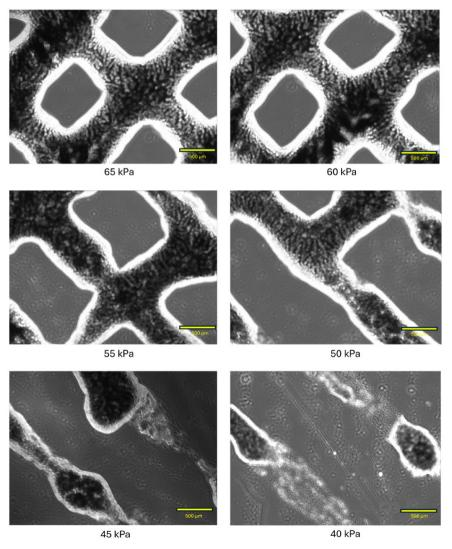
Fig. 7 Microscopic images of 7% GelMA-gelatin hydrogel under 5x magnification (scale bar – 500 μm)
