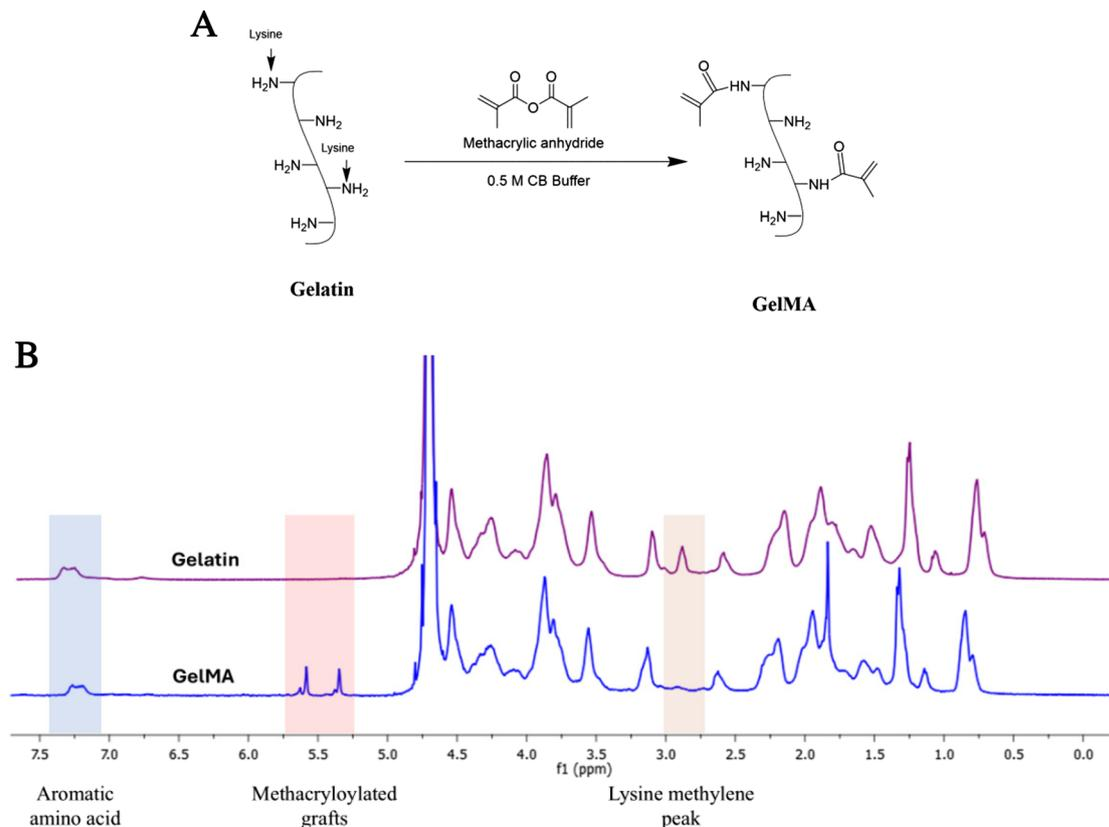
**Fig. 3** (A) Reaction of gelatin and methacrylic anhydride to form gelatin methacrylate (GelMA). (B)  $^1\text{H}$  NMR spectra of (A) unreacted gelatin and (B) GelMA obtained after the batch reaction.
