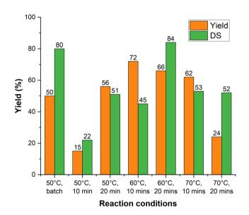
Fig. 5 Graph depicting the yield and DS% of GelMA synthesis via flow under different temperatures and residence times.
