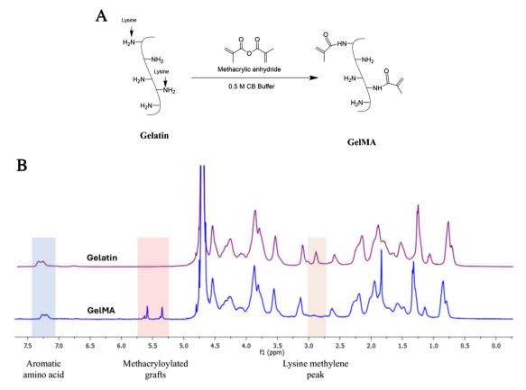
Fig. 3 (A) Reaction of gelatin and methacrylic anhydride to form gelatin methacrylate (GelMA). (B) <sup>1</sup>H NMR spectra of (A) unreacted gelatin and (B) GelMA obtained after the batch reaction.
