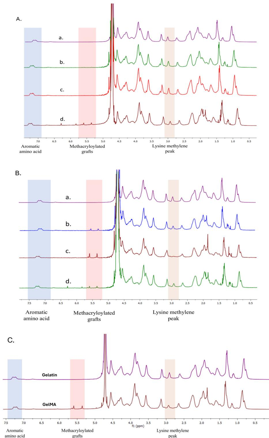
**Fig. 4** (A)  $^1\text{H}$  NMR spectra of (a) unreacted gelatin, (b) GelMA at 50 °C, (c) GelMA at 60 °C, (d) GelMA at 70 °C, at residence time of 10 min. (B)  $^1\text{H}$  NMR spectra of (a) Unreacted gelatin, (b) GelMA at 50 °C, (c) GelMA at 60 °C, (d) GelMA at 70 °C, at a residence time of 20 min. (C) GelMA synthesis reaction at 60 °C at a residence time of 20 min (highest degree of substitution) using a 6 ml reactor.
