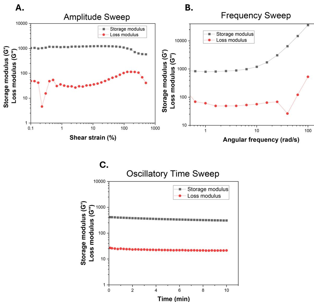
Fig. 8 Rheological analysis of GelMA-gelatin hydrogel used in bioprinting. (A) Amplitude sweep at constant frequency of  $1 \text{ rad s}^{-1}$ . (B) Frequency sweep at constant shear strain of 5%. (C) Time sweep for 10 min (shear strain 5%, frequency  $1 \text{ rad s}^{-1}$ ).
