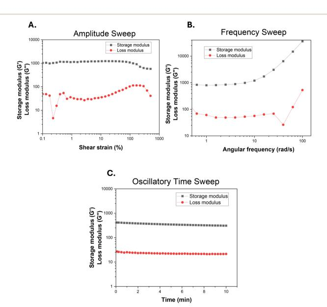
Fig. 8 Rheological analysis of GelMA-gelatin hydrogel used in bioprinting. (A) Amplitude sweep at constant frequency of 1 rad s<sup>-1</sup>. (B) Frequency sweep at constant shear strain of 5%. (C) Time sweep for 10 min (shear strain 5%, frequency 1 rad s<sup>-1</sup>).
