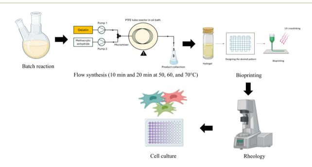
Fig. 1 Schematic representation of the experimental protocol followed in this study
