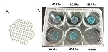
Fig. 6 (A) The desired pattern to be bioprinted with flow GelMA, generated by GeSIM Robotics software: (B) the different scaffolds bioprinted using flow GelMA with different pressures. The blue colour arises from a food dye added to aid visibility.
