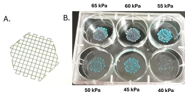
**Fig. 6** (A) The desired pattern to be bioprinted with flow GelMA, generated by GeSIM Robotics software; (B) the different scaffolds bioprinted using flow GelMA with different pressures. The blue colour arises from a food dye added to aid visibility.
