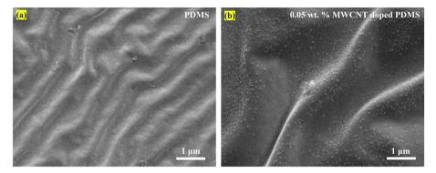
Fig. 2 SEM images of (a) pristine PDMS and (b) 0.05 wt% MWCNT-doped PDMS.
