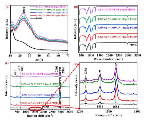
Fig. 1 Material characterization of the spin-coated PDMS-MWCNT composite membrane. (a) X-ray diffraction patterns, (b) FTIR spectra, (c) Raman spectra, and (d) enlarged view of the Raman spectra in the range from 1200 to 1800  ${\rm cm}^{-1}$ .
