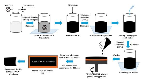
Fig. 9 Fabrication procedure for the flexible PDMS-MWCNT composite membrane
