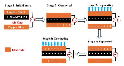
Fig. 10 Distribution of the transient charge in each tribological layer in a sequential manner, along with the operating principle of the device.
