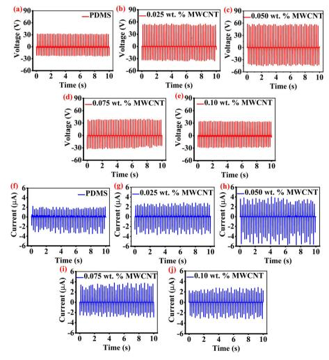
Open-circuit voltage  $(V_{oc})$  (a-e) and short-circuit current  $(I_{sc})$  (f-j) of different weight percentages of MWCNT-doped PDMS.
