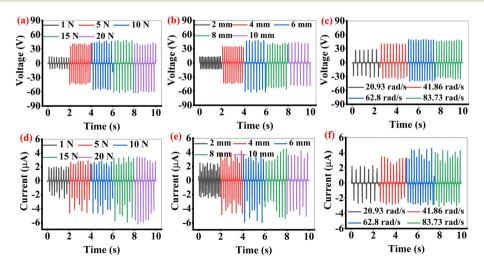
$V_{\rm oc}$  and  $I_{\rm sc}$  at different applied forces (a and d), different separation distances (b and e), and different angular velocities (c and f).
