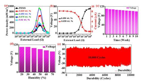
Fig. 6 (a) Power density at different load resistances for all the composite membranes, (b) impendence of PDMS-MWCNT (0.050 wt%), (c) durability test of PDMS-MWCNT (0.050 wt%) over 10 weeks, (d) effect of humidity on the output voltage, and (e) durability test for 10 000 cycles.
