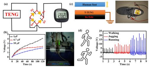
Fig. 7 Applications of TENG devices. (a) Schematic of a TENG used for charging a stopwatch, (b) demonstration of a capacitor charging using a TENG, (c) architectural design of a TENG integrated into a shoe for wearable applications, and (d) output voltage performance under different motion conditions, including walking, jogging, and running.
