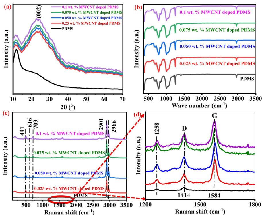
**Fig. 1** Material characterization of the spin-coated PDMS–MWCNT composite membrane. (a) X-ray diffraction patterns, (b) FTIR spectra, (c) Raman spectra, and (d) enlarged view of the Raman spectra in the range from 1200 to 1800  $\text{cm}^{-1}$ .
