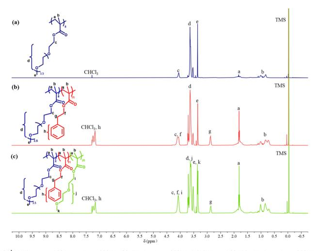
Fig. 5  $^{1}$ H NMR spectra of (a) homopolymer OEGMA<sub>8</sub>, (b) diblock polymer OEGMA<sub>8</sub>-b-PhEMA<sub>11</sub>, and (c) ABC triblock terpolymer OEGMA<sub>8</sub>-b-PhEMA<sub>11</sub>-b-DEGMA<sub>20</sub>. The chemical structures of the corresponding polymers are also shown and the different  $^{1}$ H are labelled in the spectra.
