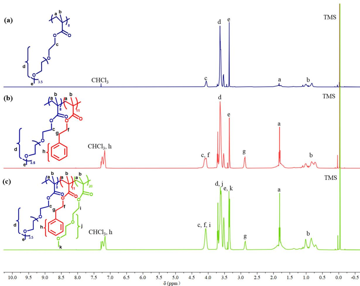
Fig. 5  $^1\text{H}$  NMR spectra of (a) homopolymer OEGMA<sub>8</sub>, (b) diblock polymer OEGMA<sub>8</sub>-*b*-PhEMA<sub>11</sub>, and (c) ABC triblock terpolymer OEGMA<sub>8</sub>-*b*-PhEMA<sub>11</sub>-*b*-DEGMA<sub>20</sub>. The chemical structures of the corresponding polymers are also shown and the different  $^1\text{H}$  are labelled in the spectra.
