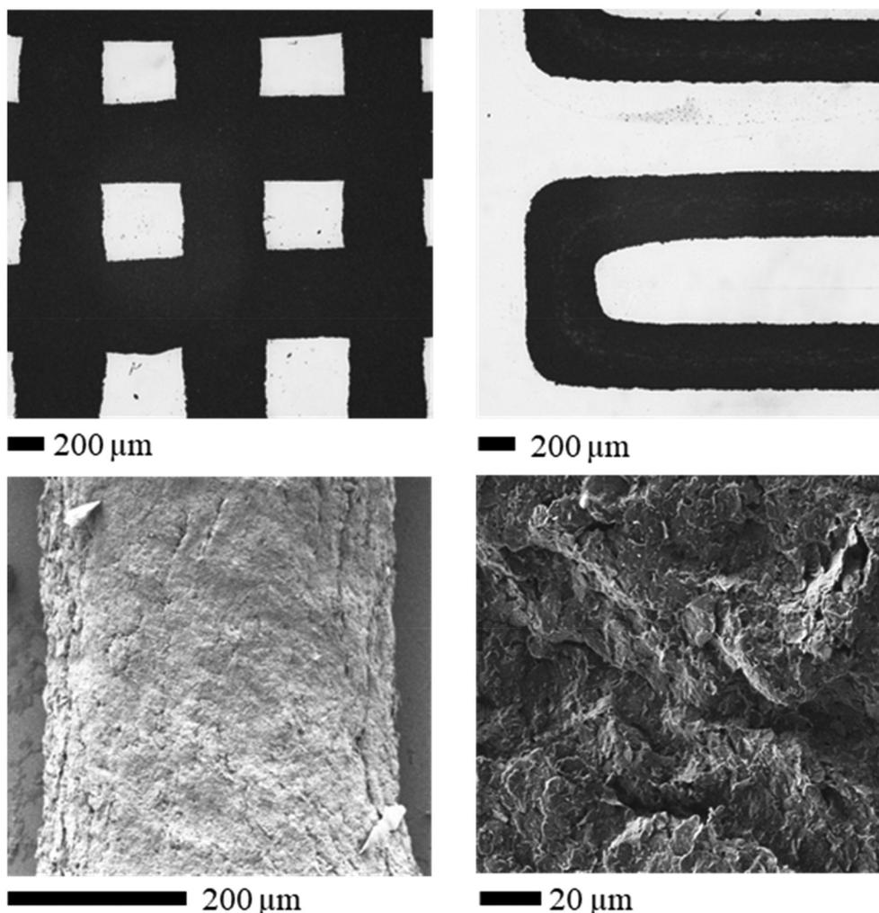
Fig. 12 SEM images of the printed structures based on 10 w/w% of P10 OEGMA<sub>10</sub>-*b*-PhEMA<sub>17</sub>-*b*-DEGMA<sub>11</sub> with 10 w/w% of graphene. (a) A two-layer cross-grid pattern, (b) a single-layer serpentine pattern, (c and d) surface morphology of the printed structure.
