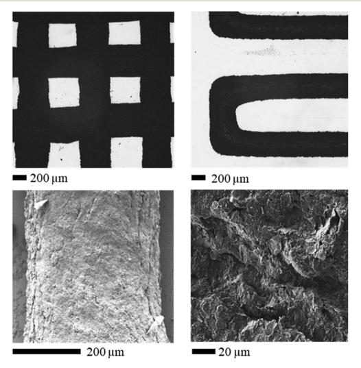
Fig. 12 SEM images of the printed structures based on 10 w/w% of P10 OEGMA<sub>10</sub>-b-PhEMA<sub>17</sub>-b-DEGMA<sub>11</sub> with 10 w/w% of graphene. (a) A twolayer cross-grid pattern, (b) a single-layer serpentine pattern, (c and d) surface morphology of the printed structure.
