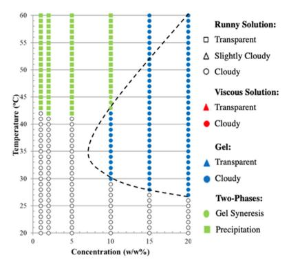
Fig. 9 A phase diagram of polymers P10 OEGMA<sub>10</sub>-b-PhEMA<sub>17</sub>-b-DEGMA<sub>11</sub> with different concentrations (1, 2, 5, 10, 15, 20 w/w%) mixed with 10 w/w% of graphene in DI water.
