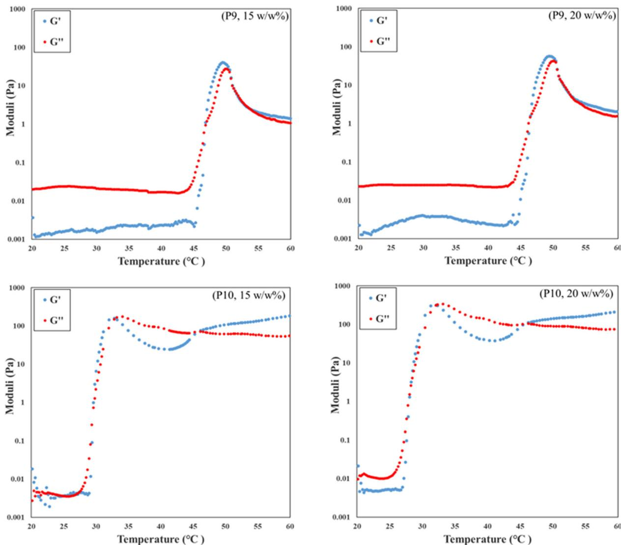
**Fig. 8** Changes of moduli (storage modulus  $G'$  is denoted by blue circles and the loss modulus  $G''$  is denoted by red circles) with temperature for the polymer solutions of P9 and P10 that can form the gel at 15 w/w% and 20 w/w% in DI water.
