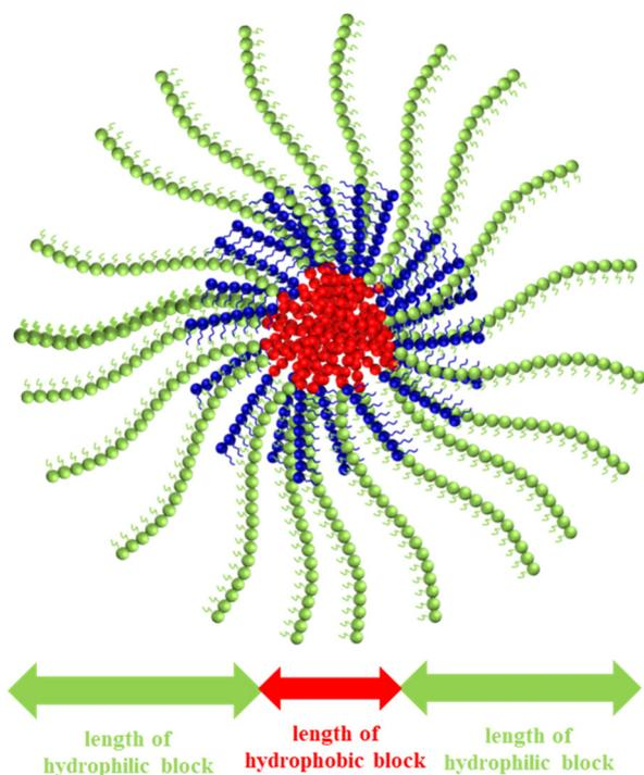
**Fig. 6** A schematic illustration of a spherical micelle with the core-shell structure of P1 OEGMA<sub>8</sub>-*b*-PhEMA<sub>11</sub>-*b*-DEGMA<sub>20</sub>. The units of OEGMA, PhEMA and DEGMA are represented in blue, red, and green spheres respectively.
