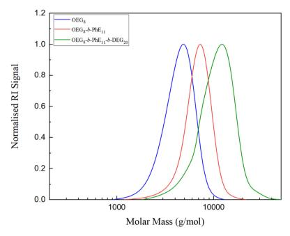
Fig. 4 The SEC traces of P1: OEGMA<sub>8</sub>-b-PhEMA<sub>11</sub>-b-DEGMA<sub>20</sub> and its precursors OEGMA<sub>8</sub> and OEGMA<sub>8</sub>-b-PhEMA<sub>11</sub> are shown in blue, red and green, respectively.
