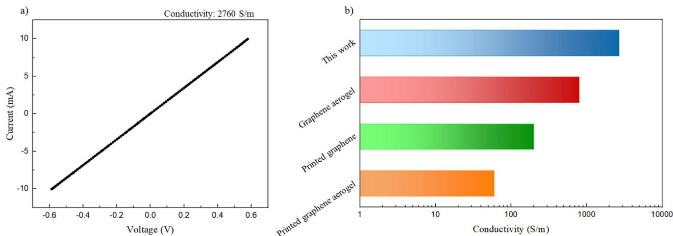
Fig. 13 (a)  $I$ - $V$  curve of the printed structure; (b) electrical conductivity of the printed structure compared with three different DIW inks.<sup>65–67</sup>
