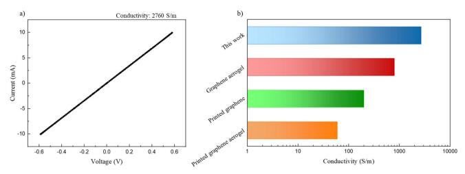
Fig. 13 (a) I–V curve of the printed structure; (b) electrical conductivity of the printed structure compared with three different DIW inks. 65–67
