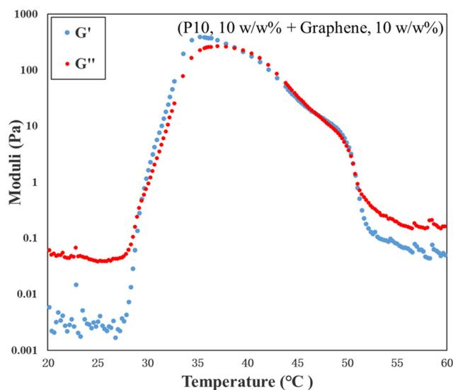
**Fig. 11** Changes of moduli (storage modulus  $G'$  is denoted by blue circles and the loss modulus  $G''$  is denoted by red circles) with temperature for the ink (10 w/w% P10 and 10 w/w% graphene in DI water).
