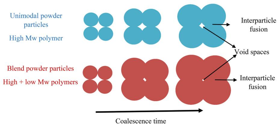
**Fig. 1** Proposed strategy to enhance coalescence and decrease void space in high  $M_w$  polymer by molecular modification. Under the same experimental condition, molecular blend sample should exhibit higher level of coalescence and lower void space than unblended samples.
