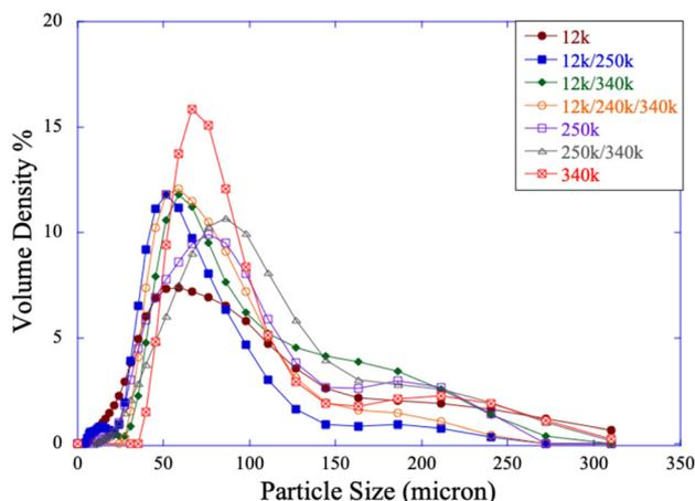
**Fig. 4** Particle size and distributions of produced PP powders analyzed using laser diffraction. The average particle size,  $D_{50}$ , is the proper size (58  $\mu\text{m}$ –86  $\mu\text{m}$ ) for PBF.
