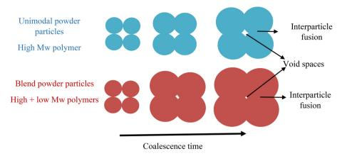
Fig. 1 Proposed strategy to enhance coalescence and decrease void space in high  $M_{\rm w}$  polymer by molecular modification. Under the same experimental condition, molecular blend sample should exhibit higher level of coalescence and lower void space than unblended samples.
