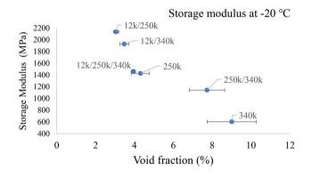
Fig. 13 Storage modulus of the printed PP part at  $-20~^{\circ}\text{C}$  as a function of void fraction.
