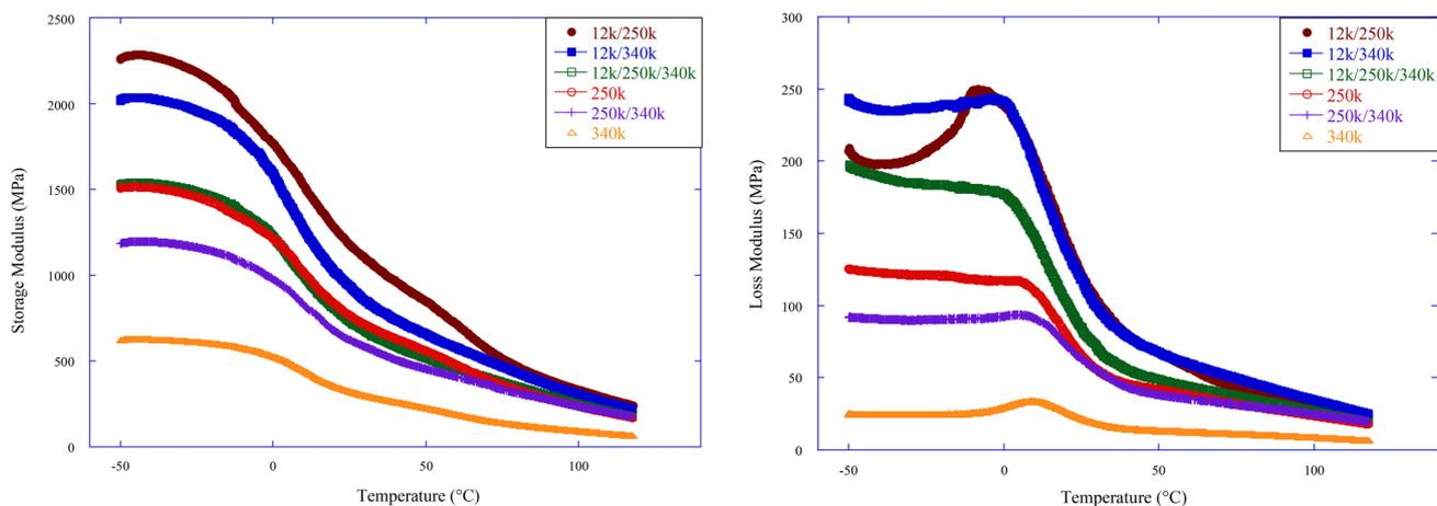
Fig. 8 Thermomechanical properties of the PP printed parts.
