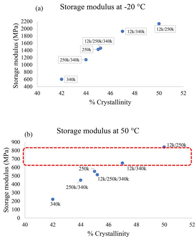
**Fig. 11** Correlation of storage modulus with PP crystallinity at  $-20\text{ }^{\circ}\text{C}$  (a) and  $50\text{ }^{\circ}\text{C}$  (b). The dashed box in (b) denotes the modulus of melt pressed PP at  $50\text{ }^{\circ}\text{C}$  as reported in Li *et al.*<sup>37</sup>
