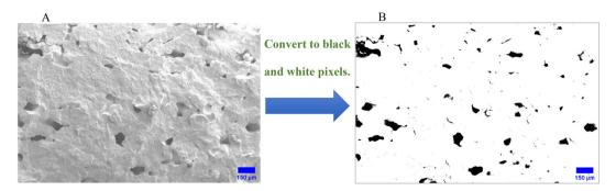
Fig. 3 Evaluation of void space in the printed sample *via* SEM and ImageJ. (A) SEM image of the printed sample showing the void spaces. (B) Converted SEM image of the printed sample to black and white pixels using ImageJ. Scale bar is 150 μm.
