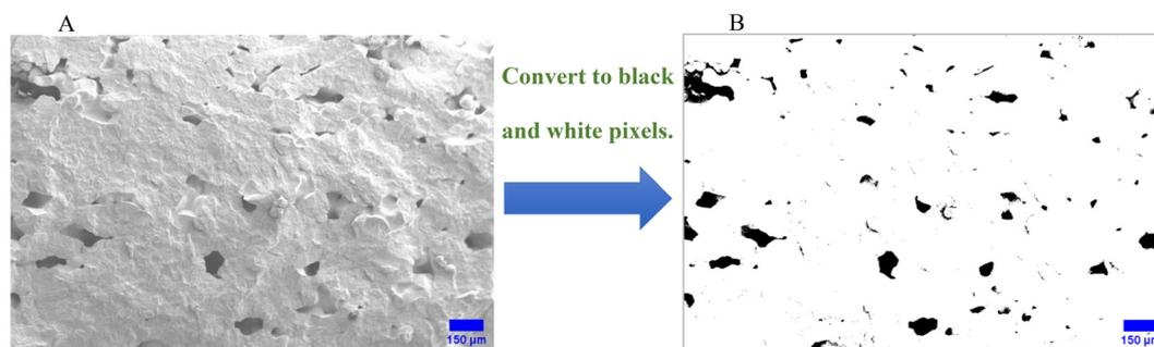
**Fig. 3** Evaluation of void space in the printed sample *via* SEM and ImageJ. (A) SEM image of the printed sample showing the void spaces. (B) Converted SEM image of the printed sample to black and white pixels using ImageJ. Scale bar is 150 μm.
