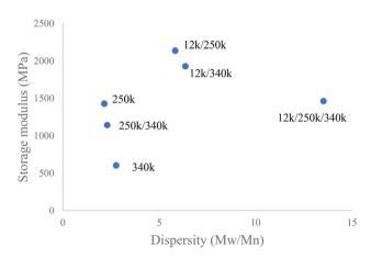
Fig. 9 The storage modulus of the printed parts at -20 °C as a function of the polymer dispersity.
