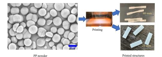
Fig. 2 Powder bed fusion of the PP powder. The tensile bars are formed from the 250K powder, while the rectangular DMA bars are formed from the 250K and 12K blend powder.
