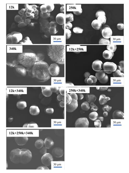
Fig. 5 Structures of PP powders obtained via scanning electron microscope. PP samples produced in this work are highly spherical. Scale bars are 30 microns.
