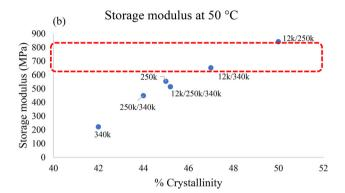
Fig. 11 Correlation of storage modulus with PP crystallinity at -20 °C (a) and 50 °C (b). The dashed box in (b) denotes the modulus of melt pressed PP at 50 °C as reported in Li *et al.*<sup>37</sup>
