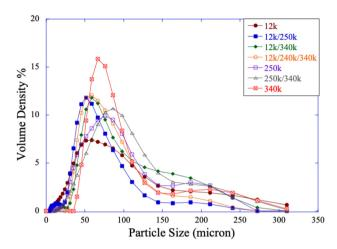
Fig. 4 Particle size and distributions of produced PP powders analyzed using laser diffraction. The average particle size, D50, is the proper size  $(58 \mu m-86 \mu m)$  for PBF.
