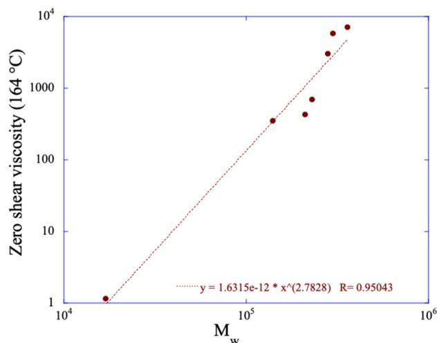
**Fig. 6** Zero shear viscosities of PP powders as a function of weight average molecular weight of the polymers.
