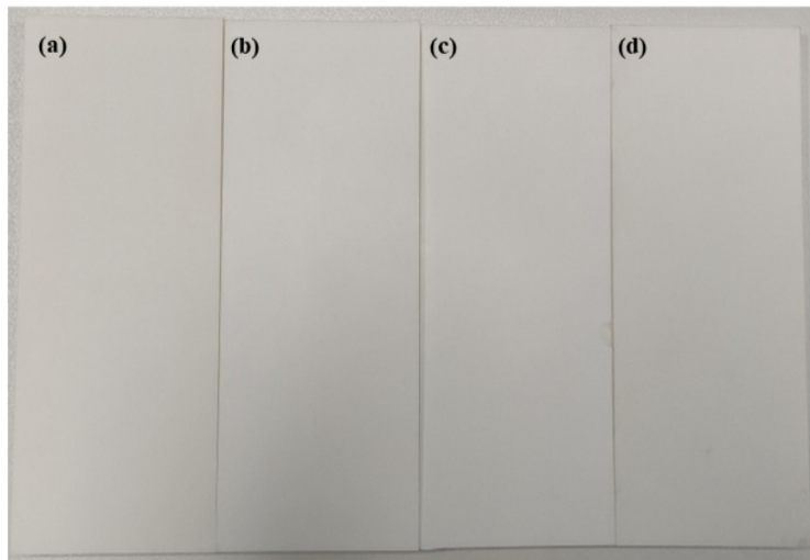
Fig. 7 Different types of ultraviolet absorbers added to acrylic adhesive different color difference performance. (a) Blank, the value of \Delta E is 4.55. (b) Basf 329 UV absorber was added, the value of \Delta E is 24.39. (c) Basf 326 UV absorber was added, the value of \Delta E is 23.63. (d) Added Chick 2912 UV absorber, the value of \Delta E is 5.28.
