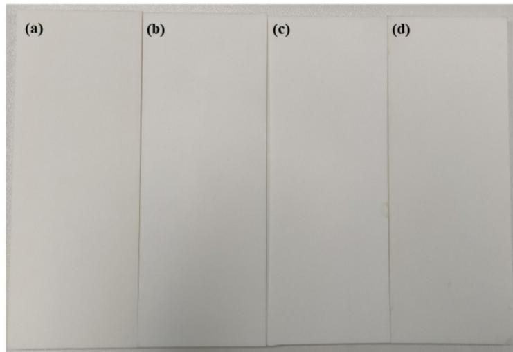
**Fig. 7** Different types of ultraviolet absorbers added to acrylic adhesive different color difference performance. (a) Blank, the value of  $\Delta E$  is 4.55. (b) Basf 329 UV absorber was added, the value of  $\Delta E$  is 24.39. (c) Basf 326 UV absorber was added, the value of  $\Delta E$  is 23.63. (d) Added Chick 2912 UV absorber, the value of  $\Delta E$  is 5.28.
