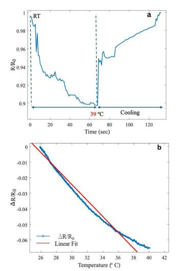
Fig. 4 (a) Normalized resistance of the temperature sensor on fabric versus time for one heating and cooling cycle and (b) sensitivity of the sensor with temperature and a linear fit to the results.
