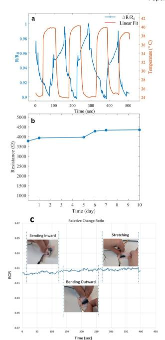
Fig. 5 Dynamic response of the sensor showing  $R/R_0$  and reference temperature over multiple cycles. (b) Long-term stability at 36 °C over 10 days, with a 13% resistance increase due to fabric stretching. (c) Relative Change Ratio (RCR) of the sensor under bending inward, bending outward, and stretching.
