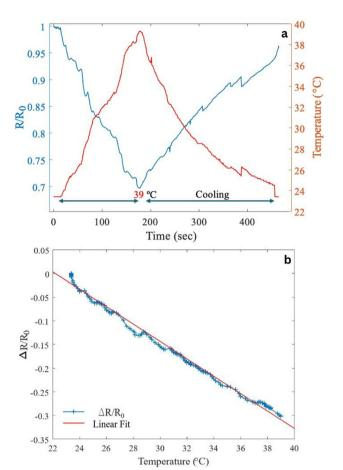
Fig. 3 (a) Normalized resistance of the temperature sensor on glass versus time for one heating and cooling cycle and (b) sensitivity of the sensor with temperature and a linear fit to the results.
