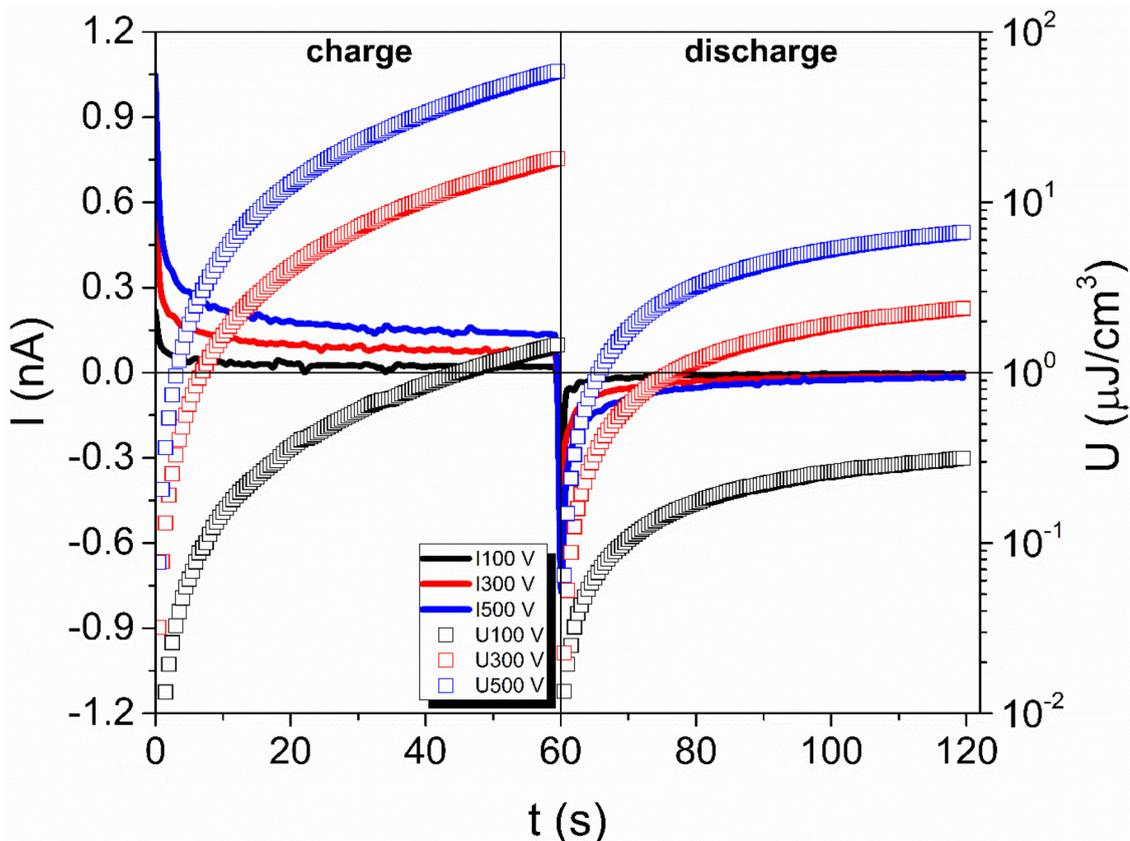
Fig. 6 The measured charge/discharge currents and the calculated stored/recovered energy densities are presented as a function of time, varying the applied dc voltage during charging for  $e_{96}(\text{PVA5}:1\text{CS})f_4$ .
