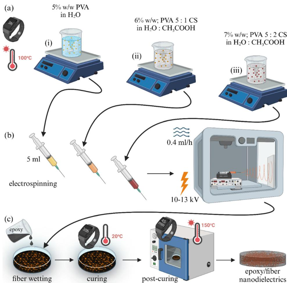
**Fig. 1** Schematic representation of the sample preparation steps, namely: (a) polymer/solvent solutions where (i) plain PVA, (ii) PVA 5 : 1 CS, and (iii) PVA 5 : 2 CS; (b) filler electrospinning; and (c) incorporation of electrospun nanofibrous membranes into the epoxy resin. Created with BioRender.com.
