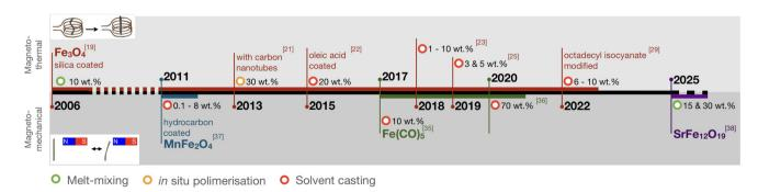
Fig. 1 Chronological overview of magnetic soft actuators, produced with a TPU matrix. The timeline is divided distinguishing between magnetothermal (top) and magnetomechanical (bottom) actuation mechanisms. Open circles, in different colours, denote the different processing methods.
