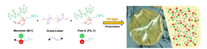
Fig. 2 Illustration of composite poly(IL)-IL membrane preparation. Photograph on the right shows a freestanding membrane held in a gloved hand.
