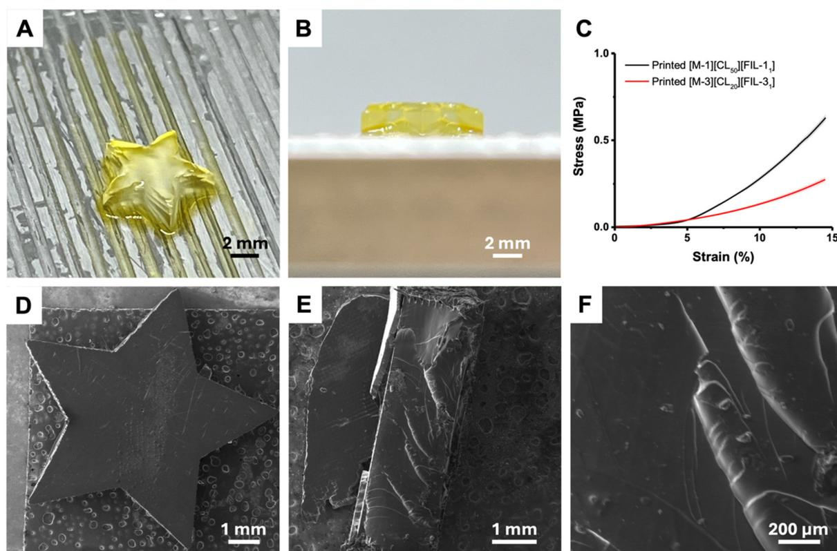
**Fig. 5** Images of [M-1][CL<sub>50</sub>][FIL-1<sub>1</sub>] printed by digital light processing (DLP): (A) on build platform from the top and (B) from the side. (C) Stress-strain curve from the DMA compression test of both [M-1][CL<sub>50</sub>][FIL-1<sub>1</sub>] and [M-3][CL<sub>20</sub>][FIL-3<sub>1</sub>]. SEM images: (D) top view, (E) cross-section, and (F) cross-section magnification.
