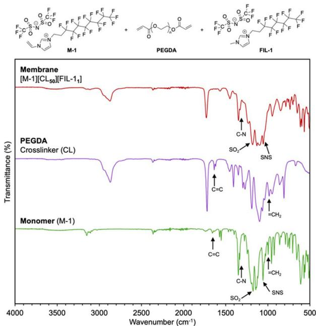
Fig. 3 FTIR spectra of M-1, PEGDA, and poly(IL)-IL membrane [M-1][CL<sub>50</sub>][FIL-1<sub>1</sub>].
