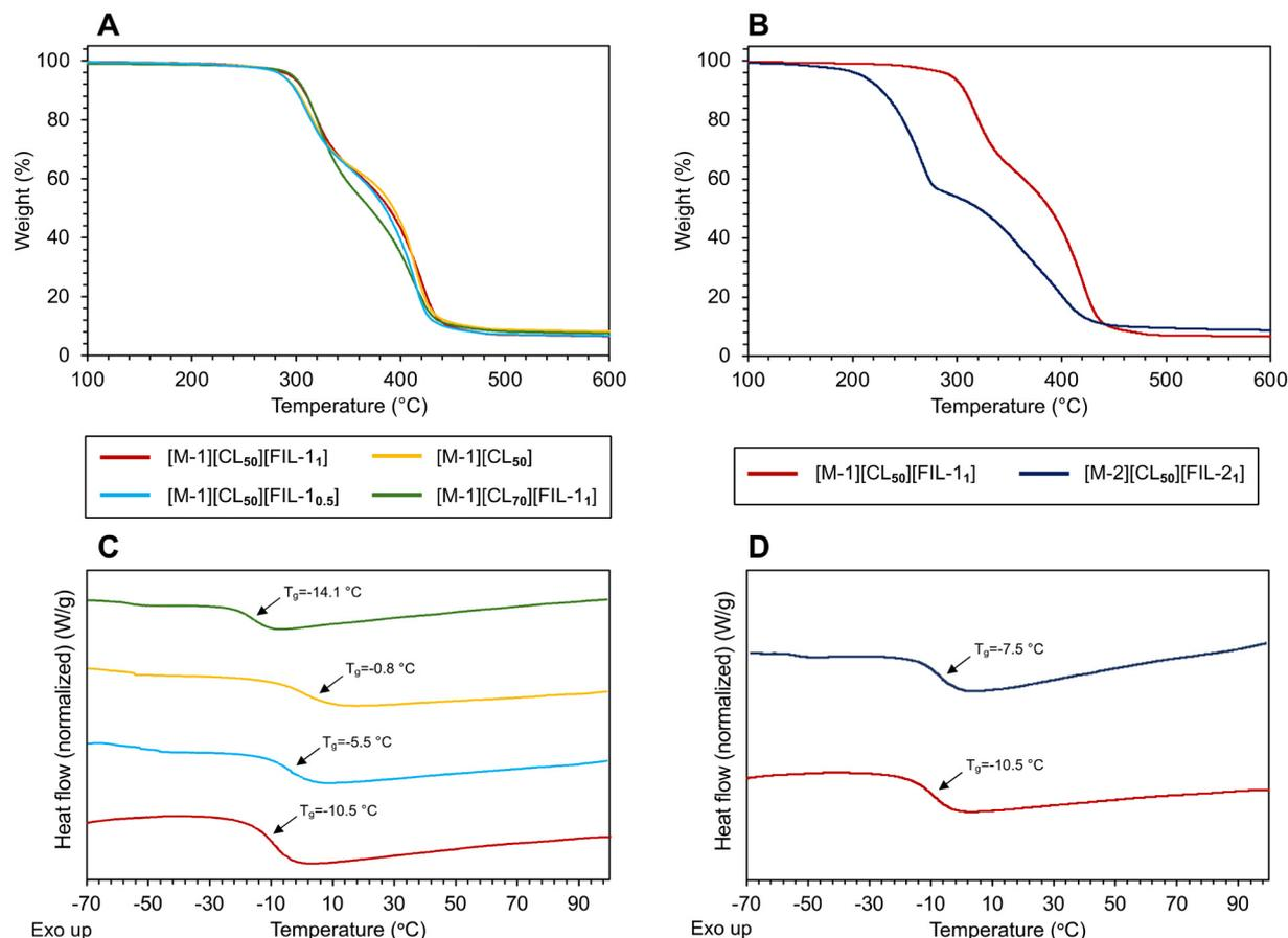
**Fig. 4** (A) Thermal weight loss profiles of membranes prepared from M-1. (B) Comparison of thermal weight loss profile of [M-1][CL<sub>50</sub>][FIL-1<sub>1</sub>] and [M-2][CL<sub>50</sub>][FIL-2<sub>1</sub>]. (C) Second heating cycle of the DSC thermogram of poly(IL)-IL membranes prepared from M-1. (D) Second heating cycle of the DSC profile comparing [M-1][CL<sub>50</sub>][FIL-1<sub>1</sub>] and [M-2][CL<sub>50</sub>][FIL-2<sub>1</sub>].
