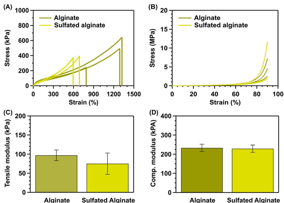
**Fig. 5** Strength and modulus comparison of the control vs. sulfated alginate hydrogels, synthesized via the one-step method. (A) Tensile stress-strain curves of the control and sulfated alginate 2A hydrogels. (B) Compressive stress-strain curves of the control and sulfated alginate 2A hydrogels. (C) Tensile modulus of the control and sulfated alginate 2A hydrogels. (D) Compressive (comp.) modulus of the control and sulfated alginate 2A hydrogels.
