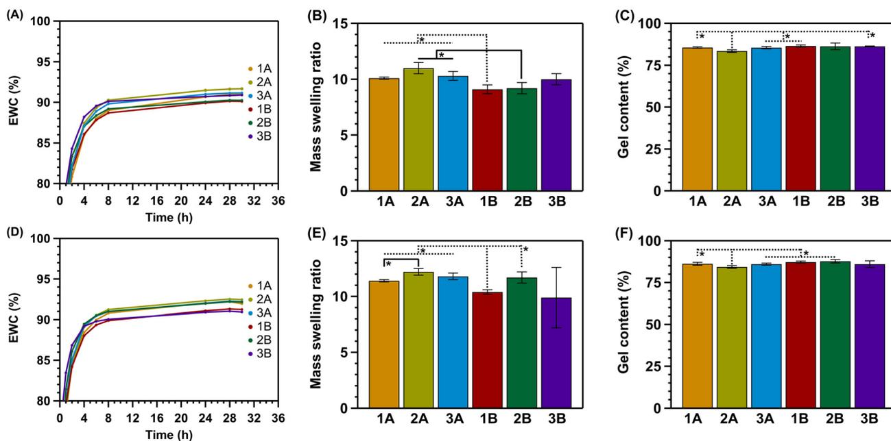
Fig. 3 Swelling tests of the one-step solution gel-method hydrogels. (A–C) Equilibrium water content, mass swelling ratio, and gel content of all six hydrogel formulations synthesized *via* the one-step method, swollen at RT = 23 °C, respectively. (D–F) Equilibrium water content, mass swelling ratio, and gel content of all six hydrogel formulations synthesized *via* the one-step method, swollen at 37 °C, respectively. Significant differences at indicated \* ( $p < 0.05$ ).
