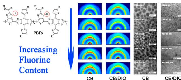
**Fig. 4** Molecular structure, GIXD scattering images of PBFx polymers and blends and TEM images of PBFx:PCBM blends. Reprinted (adapted) with permission from ref. 46. Copyright 2014 American Chemical Society.
