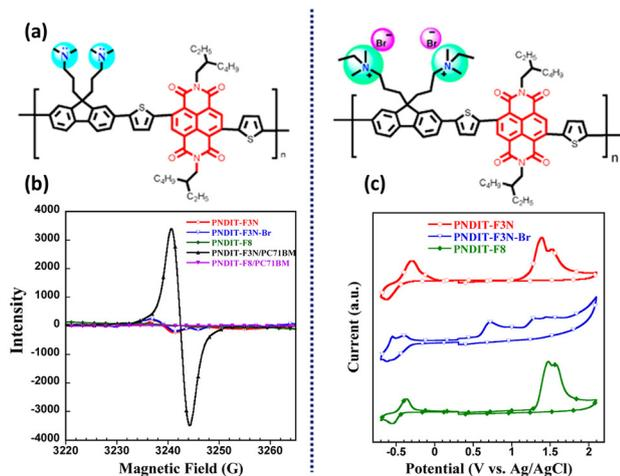
**Fig. 13** (a) Chemical structures of PNDIT-F3N and PNDIT-F3N-Br. (b) ESR spectra of different polymers and blends in solid state. (c) Cyclic voltammograms of the polymers. Reprinted (adapted) with permission from ref. 124. Copyright 2016 American Chemical Society.
