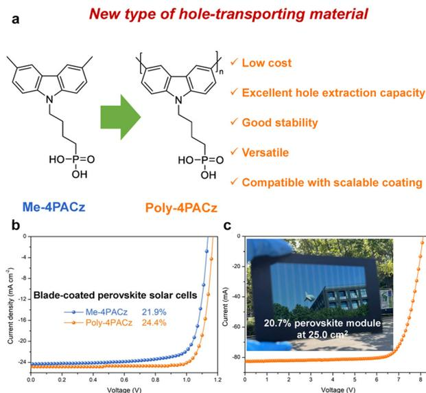
**Fig. 19** (a) Molecular structure of Me-4PACz and Poly-4PACz. (b)  $J$ – $V$  curves of the blade-coated PSCs based on Me-4PACz and Poly-4PACz. (c)  $J$ – $V$  characteristics of the Poly-4PACz-based perovskite mini-module with an aperture area of 25.0 cm<sup>2</sup>. Inset shows a picture of Poly-4PACz-based perovskite module.
