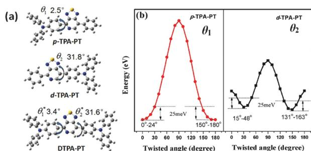
**Fig. 6** (a) DFT-optimized geometries and D–A twist angles of p-TPA-PT, d-TPA-PT, and DTPA-PT. (b) The ground-state energies of p-TPA-PT, d-TPA-PT at different D–A torsion angles in the gas phase, using the cam-b3lyp method and a full geometrical optimization at each twist angle.<sup>60</sup>
