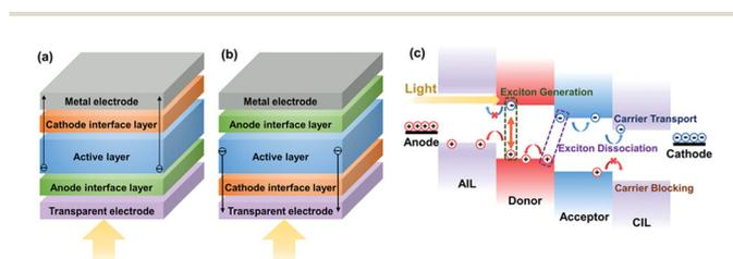
**Fig. 15** The structure of single-junction OSCs and working mechanism illustration. OSC devices in (a) conventional structure or (b) inverted structure. (c) The working mechanism of carrier generation and transport in OSCs.<sup>1</sup>
