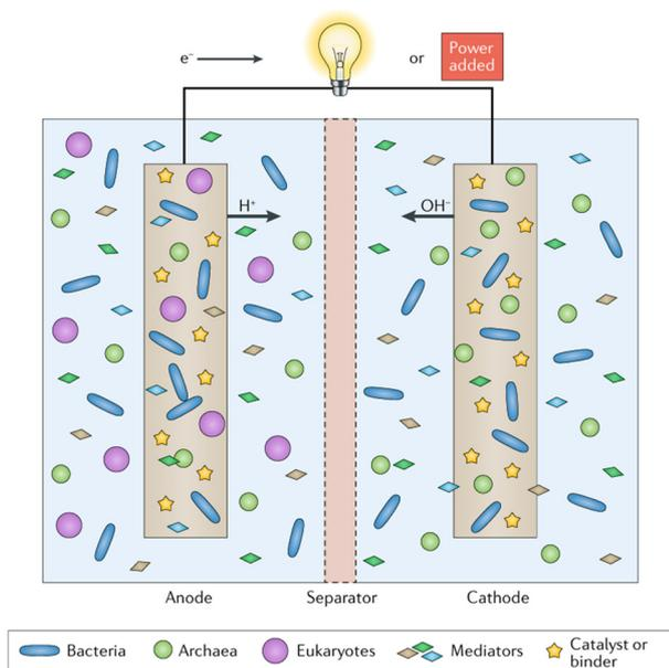
**Fig. 28** Components of microbial fuel cells and other bioelectrochemical systems.<sup>256</sup>
