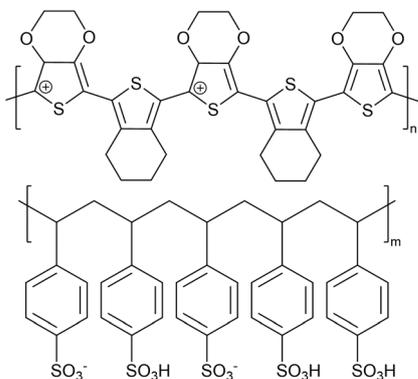
Fig. 10 (a) Chemical structures of PEDOT and PSS.
