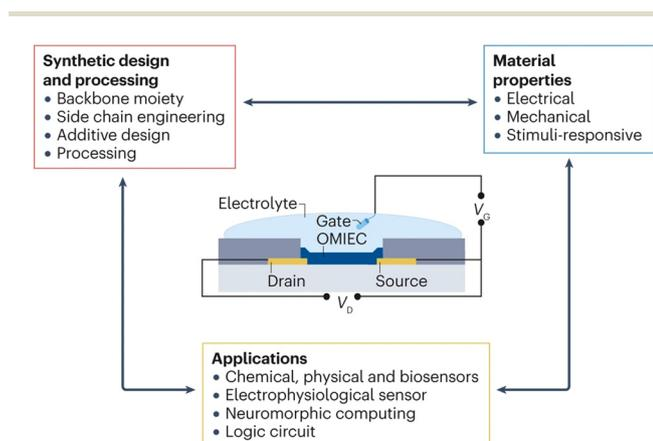
**Fig. 22** The synthetic design controls the properties of organic mixed ionic–electronic conductors (OMIECs), which enable particular applications.<sup>31</sup>
