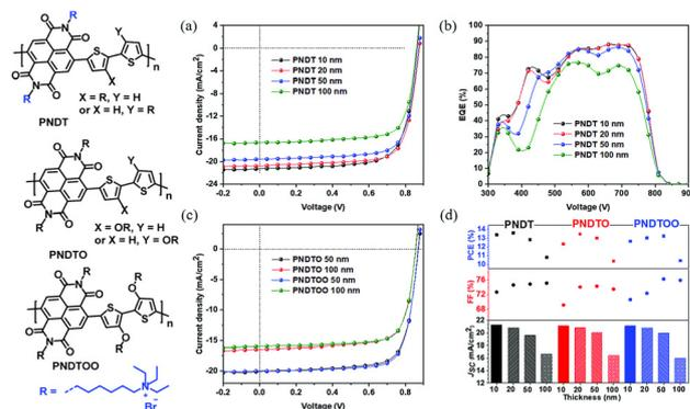
**Fig. 20**  $J$ - $V$  characteristics (a) and (b) the EQE curves of PBDB-2Cl:ITIC-2F-based photovoltaic devices with PNDT as the ETM; (c)  $J$ - $V$  characteristics of PBDB-2Cl:ITIC-2F-based photovoltaic devices with PNDTO and PNDTOO as ETMs; and (d) the summary of photovoltaic parameters for PBDB-2Cl:ITIC-2F-based photovoltaic devices with these CPEs as ETMs.<sup>122</sup>
