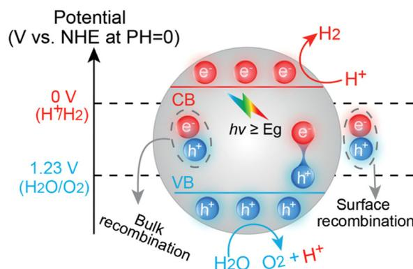
**Fig. 26** The schematic process of photocatalytic mechanism.<sup>251</sup>
