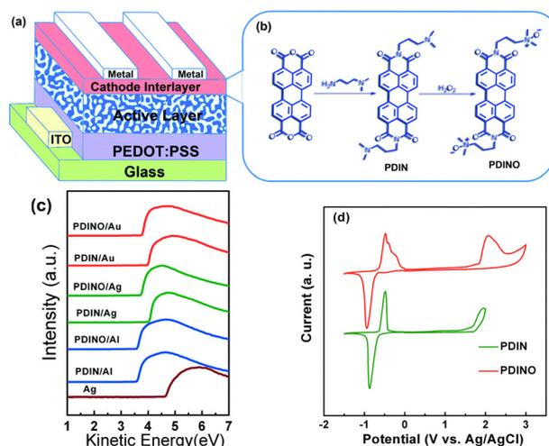
**Fig. 12** (a) Device structure of the PSCs. (b) Synthetic route towards PDI-interlayers. Device parameters of the PSCs based on PTB7/PC<sub>70</sub>BM with PDI/Al as the cathode with various PDI thicknesses under the illumination of AM 1.5 G,  $100 \text{ mW cm}^{-2}$ . (c) UPS spectra of the PDI-interlayer treated electrodes. (d) Cyclic voltammograms of the PDIs.<sup>123</sup>
