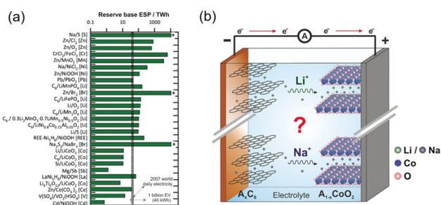
**Fig. 23** (a) Energy storage potential in TWh for different battery chemistries. The limiting element by resource constraints is shown in brackets. The star indicates that the ESP value is beyond the limit of the Figure. (b) Sketch of the well-known working principle of a lithium-ion battery (LIB) with lithium ions intercalating into two host structures.<sup>223</sup>
