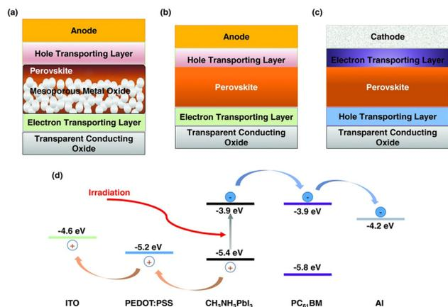
**Fig. 16** (a) Schematic diagram of regular mesoporous structure, (b) schematic diagram of regular planar structure, (c) schematic diagram of inverted planar structure, (d) schematic diagram of the working principle in the inverted Pero-SC.<sup>151</sup>
