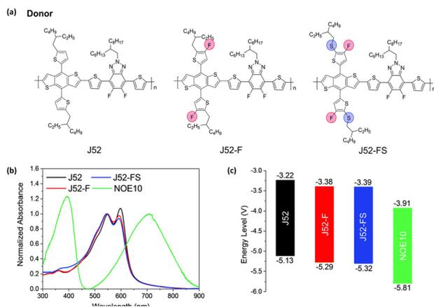
**Fig. 8** (a) Molecular structures of copolymers. (b) Optical absorption spectra of thin films; (c) energy level diagram of J52, J52-F, J52-FS, and NOE10.<sup>69</sup>
