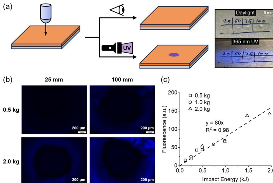
**Fig. 3** Detection of impact damage by mechanochemical fluorescence. (a) The impact experiments to quantify the effect of impact on mechanochemical fluorescence response in mechanophore-containing coatings. (b) Fluorescence microscopic images of the impact areas of the clear coating that was struck by a falling punch of two different weights and from two different heights. Scale bar = 200  $\mu\text{m}$ . (c) The profile of change in fluorescence intensity as a function of the impact energy.
