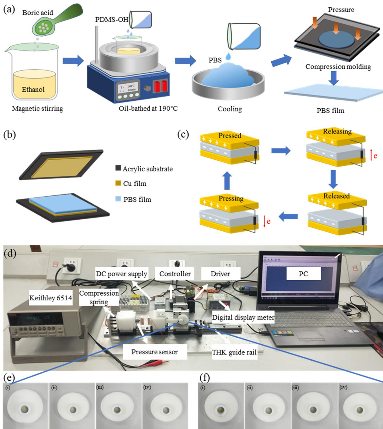
**Fig. 1** (a) Schematic diagram of the PBS film preparation process; (b) schematic diagram of a TENG based on PBS films; (c) schematic showing the contact-separation mode; (d) contact-separation mode triboelectric performance test platform; (e) cams with different follower motion profiles: (i) constant velocity, (ii) constant acceleration, (iii) simple harmonic motion, and (iv) cycloidal motion; and (f) cams with different dwell angles: (i) 30°, (ii) 60°, (iii) 90°, and (iv) 120°.
