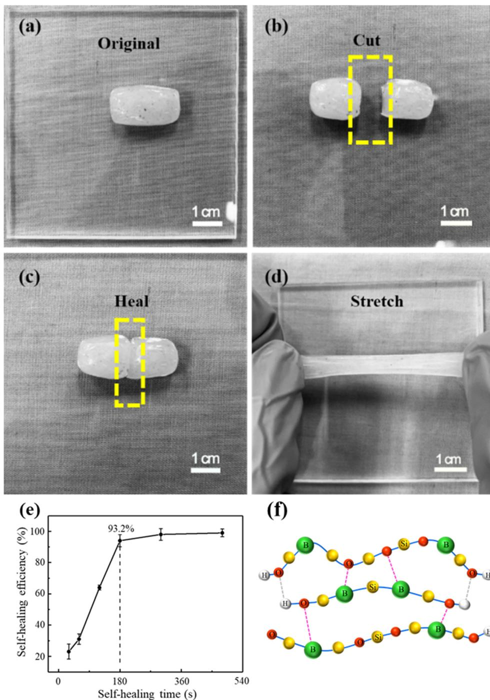
**Fig. 4** Self-healing process of PBS: (a) initial state; (b) severed; (c) healed; (d) stretched; (e) relationship between self-healing efficiency and time; and (f) schematic diagram of the internal cross-linking structure of PBS.
