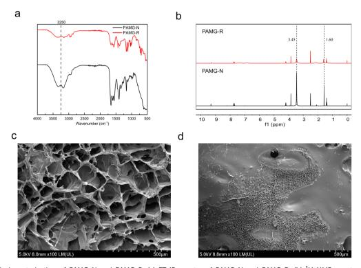
Fig. 4 Structural characterization of PAMG-N and PAMG-R. (a) FT-IR spectra of PAMG-N and PAMG-R; (b) <sup>1</sup>H NMR spectra of PAMG-N and PAMG-R; (c) SEM image of PAMG-N; (d) SEM image of PAMG-R.
