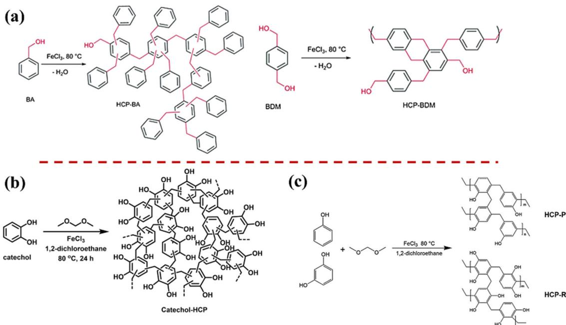
Fig. 8 (a) Synthesis of HCP-BA and HCP-BDM based on a Friedel–Crafts alkylation reaction catalyzed self-condensation.<sup>130</sup> Copyright 2013, The Royal Society of Chemistry. (b) The scheme of catechol-based HCP.<sup>53</sup> Copyright 2020, Springer. (c) Fabrication of hypercrosslinked hydroxyl-rich polymer (HCP-P and HCP-R).<sup>56</sup> Copyright 2020, Elsevier.
