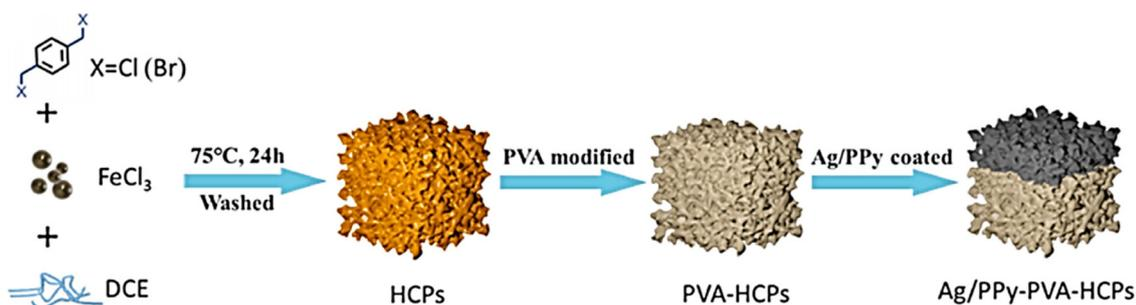
Fig. 3 Synthesis of DCX-based hypercrosslinked polymer and its functionalization.<sup>99</sup> Copyright 2021, Elsevier.
