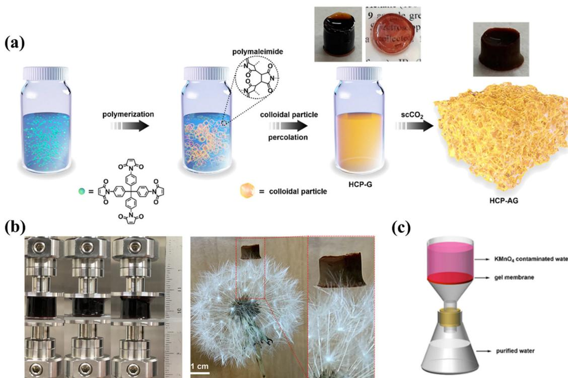
**Fig. 13** (a) Synthesis of HCP gels and aerogels via gelation processes. (b) Photographs of HCP gels and aerogels. (c) The gel membrane separation system.<sup>144</sup> Copyright 2022, American Chemical Society.
