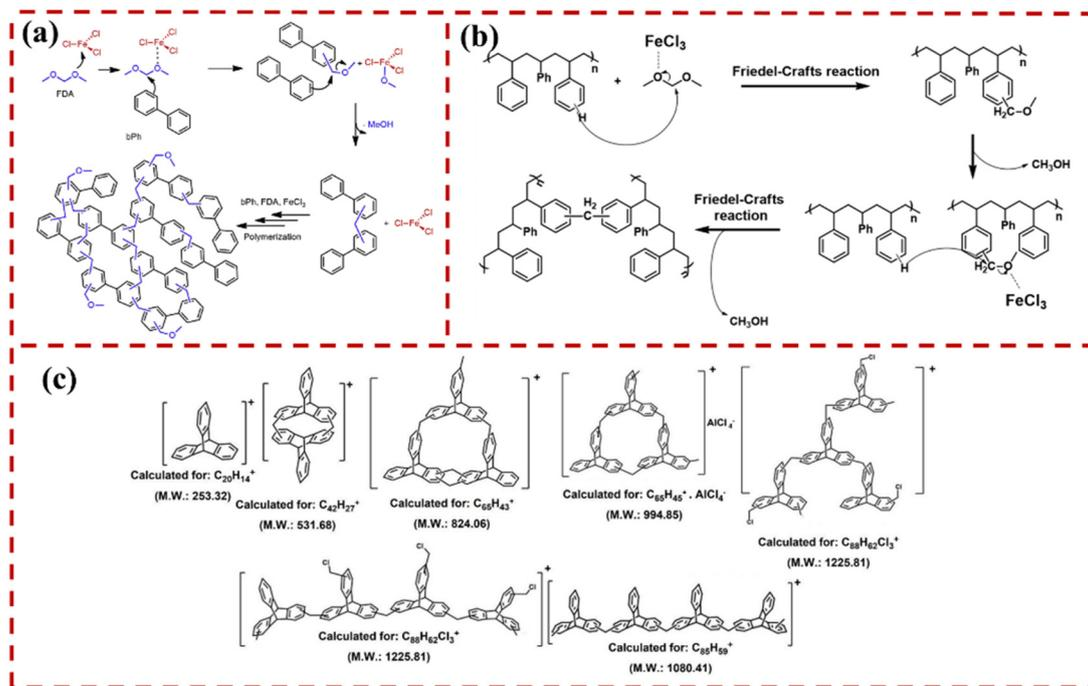
Fig. 1 (a) Synthesis pathway: polymerization of HCP via FDA as crosslinker.<sup>45</sup> Copyright 2021, Elsevier. (b) Proposed mechanism of polystyrene-based hypercrosslinked polymer.<sup>46</sup> Copyright 2020, Elsevier. (c) Solvent knitting polymerization: MALDI-TOF analysis of the samples obtained after 30 min.<sup>47</sup> Copyright 2022, American Chemical Society.
