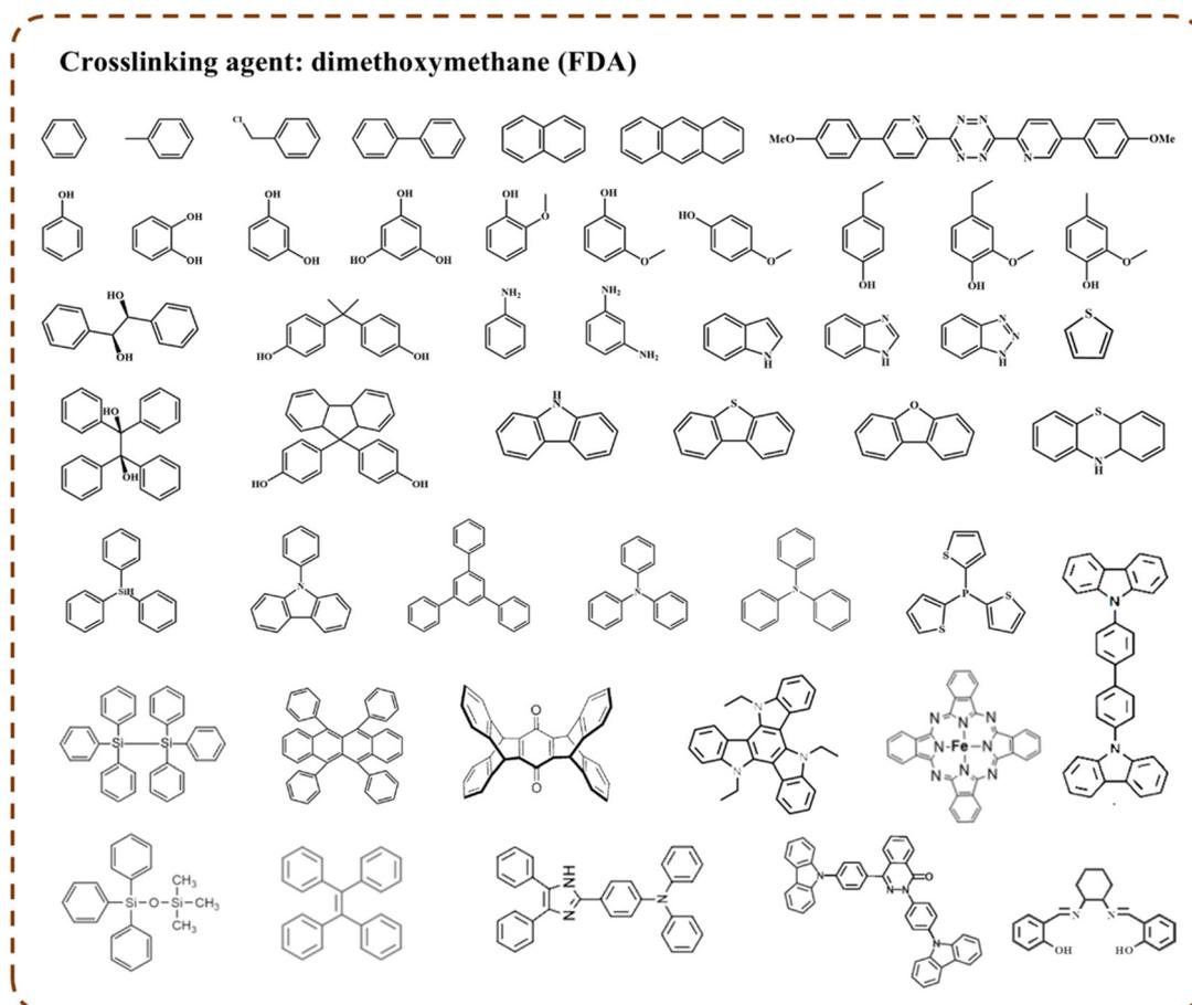
Fig. 2 Monomers for external crosslinking reaction (1,2-dichloroethane as solvent, FDA as crosslinking agent, FeCl<sub>3</sub> as catalyst).
