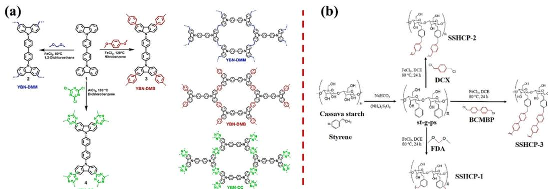
**Fig. 4** (a) Synthesis of three microporous polymers by using dicarbazole building blocks with different crosslinkers.<sup>78</sup> Copyright 2020, Elsevier. (b) Synthetic strategy of SSHCPs with some typical external crosslinkers containing biphenyl, methylene, and xylene, respectively.<sup>58</sup> Copyright 2021, Elsevier.
