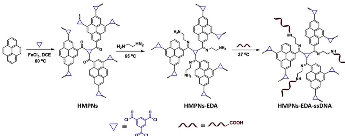
**Fig. 5** Synthesis of hypercrosslinked microporous polymer nanospheres (HMPNs) based on a Friedel–Crafts reaction by using pyrene as monomer and 1,3,5-benzenetricarbonyl trichloride as crosslinker.<sup>120</sup> Copyright 2022, Elsevier.
