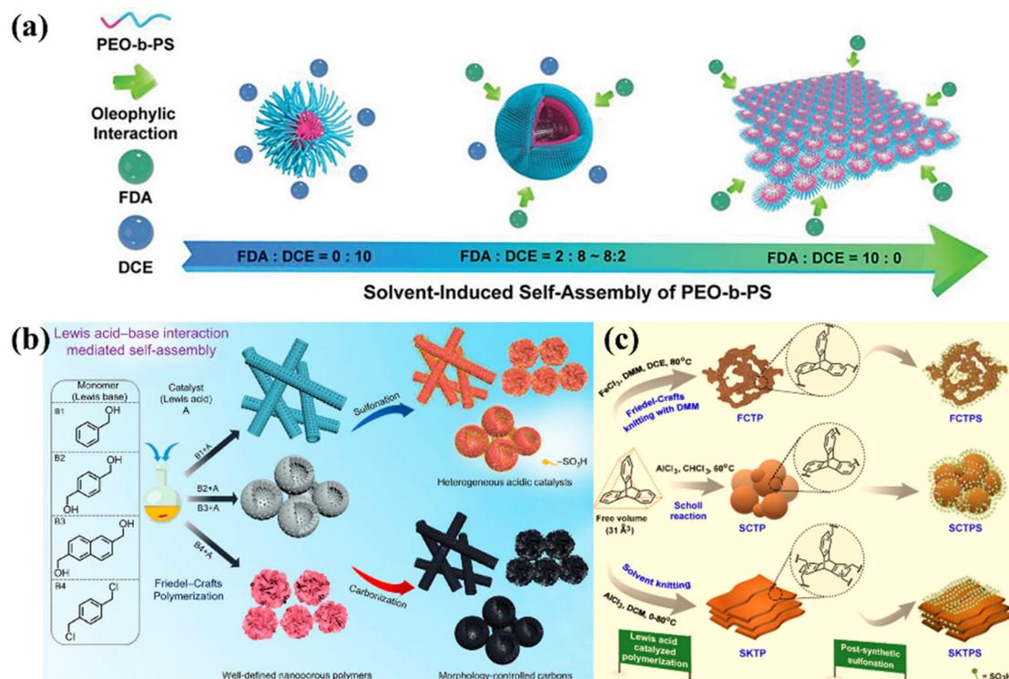
**Fig. 11** (a) Solvent-induced self-assembly strategy to produce PEO-*b*-PS-based porous polymers.<sup>134</sup> Copyright 2019, Wiley-VCH. (b) Synthesis processes of hierarchical nanoporous polymers *via* the Friedel-Crafts reaction polycondensation.<sup>135</sup> Copyright 2019, American Chemical Society. (c) Synthesis of SCTPS through a Scholl reaction using chloroform at 60 °C for 24 h.<sup>47</sup> Copyright 2022, American Chemical Society.
