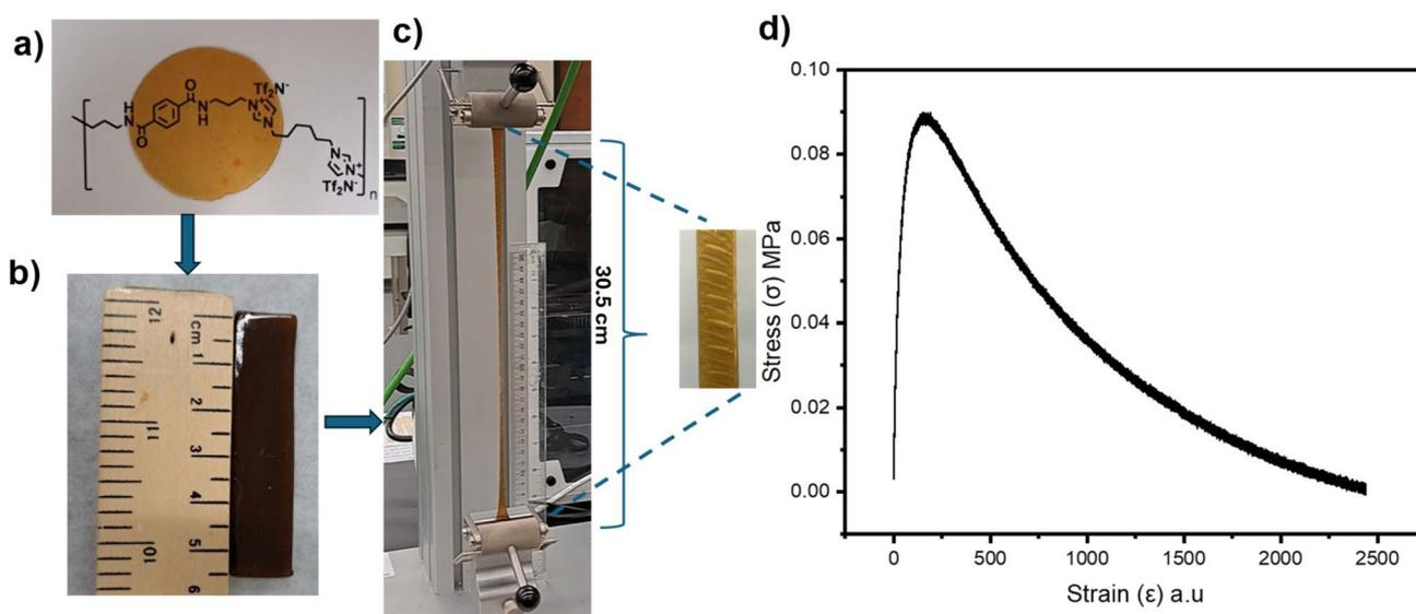
Fig. 4 (a) A thin film prepared from 3A1P-im PA-ionene at RT. (b) 3D-printed slab specimen made *via* FDM at 170 °C (10 layers, 3.2 mm total thickness). (c) Tensile testing of the slab showing high elongation at break. (d) Stress–strain plot of the resultant stress.
