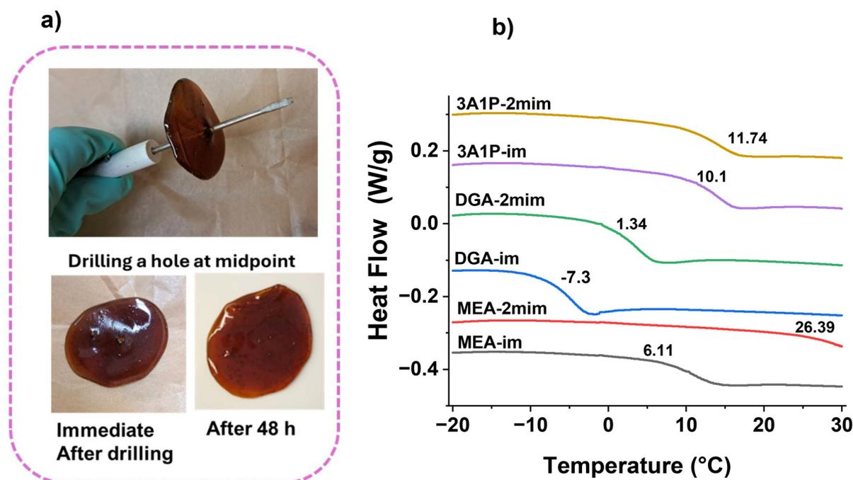
Fig. 3 (a) Self-healing of a thick film prepared from PET-derived PA ionene, DGA-2mim. (b) DSC thermograms for all six PA ionenes.
