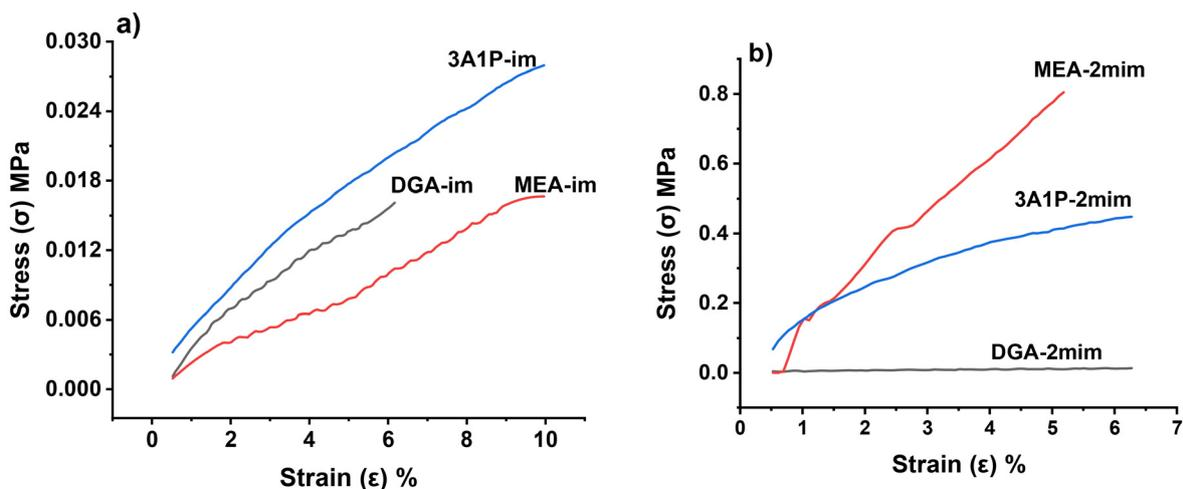
Fig. 6 Representative modulus of elasticity ( $\epsilon$ ) from stress–strain curves for PA-ionenes with (a) C(2)–H imidazolium cations and (b) C(2)–CH<sub>3</sub> imidazolium cations.
