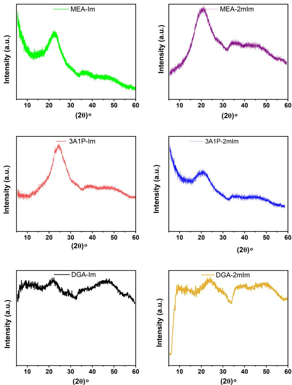
Fig. 2 XRD profiles for six separate PA-ionene materials (left =  $C_6$ -im<sub>2</sub>, right =  $C_6$ -mim<sub>2</sub>). Top: MEA. Middle: 3A1P. Bottom: DGA.
