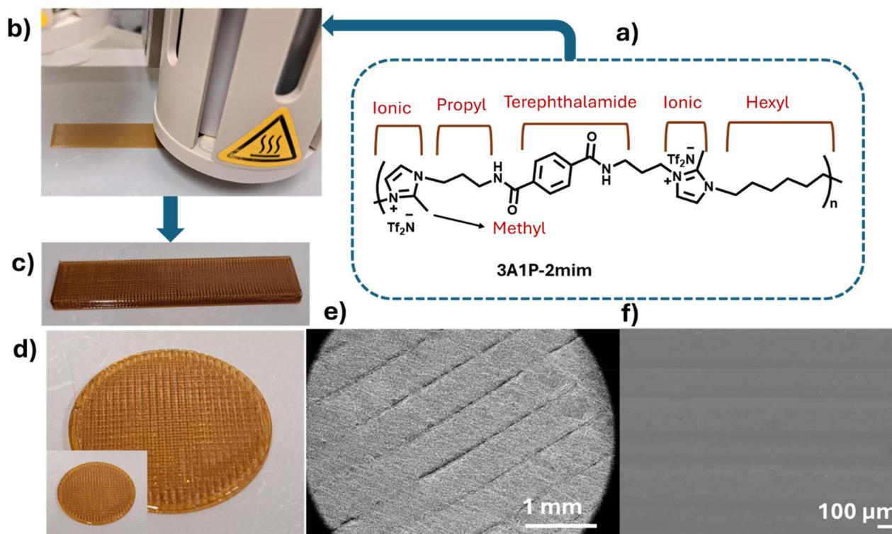
**Fig. 5** (a) Repeat unit structure and segments of 3A1P-2mim PA-ionene contributing intramolecular interaction. (b) 3D printing of first two layers of a slab (~0.66 mm thickness at this point). (c) Completed slab (9 layers, ~2.88 mm thickness). (d) 3D printed disc (5 layers, 1.2 mm thickness). (e) SEM infill pattern orientation for 3D printed slabs and discs. (f) Stretching was observed in the SEM image of the slab after tensile testing.
